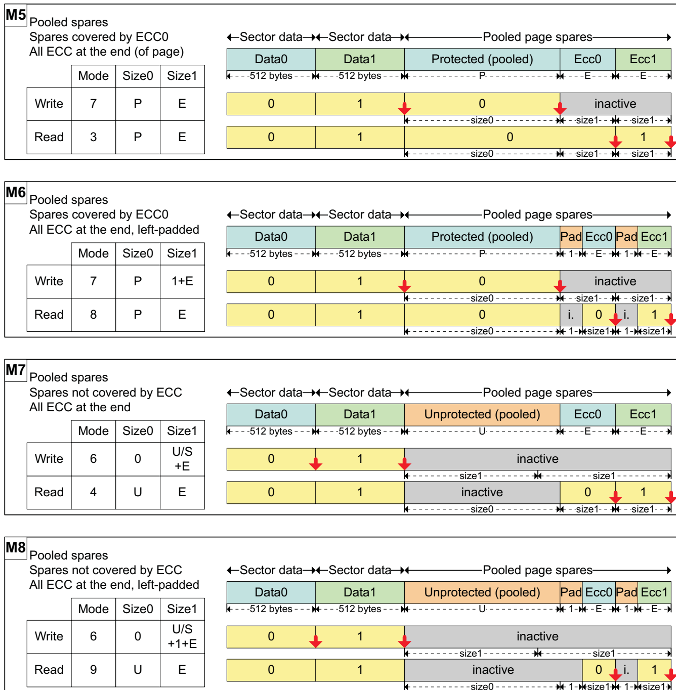
Figure 10-34. NAND Page Mapping and ECC: Pooled Spare Schemes
