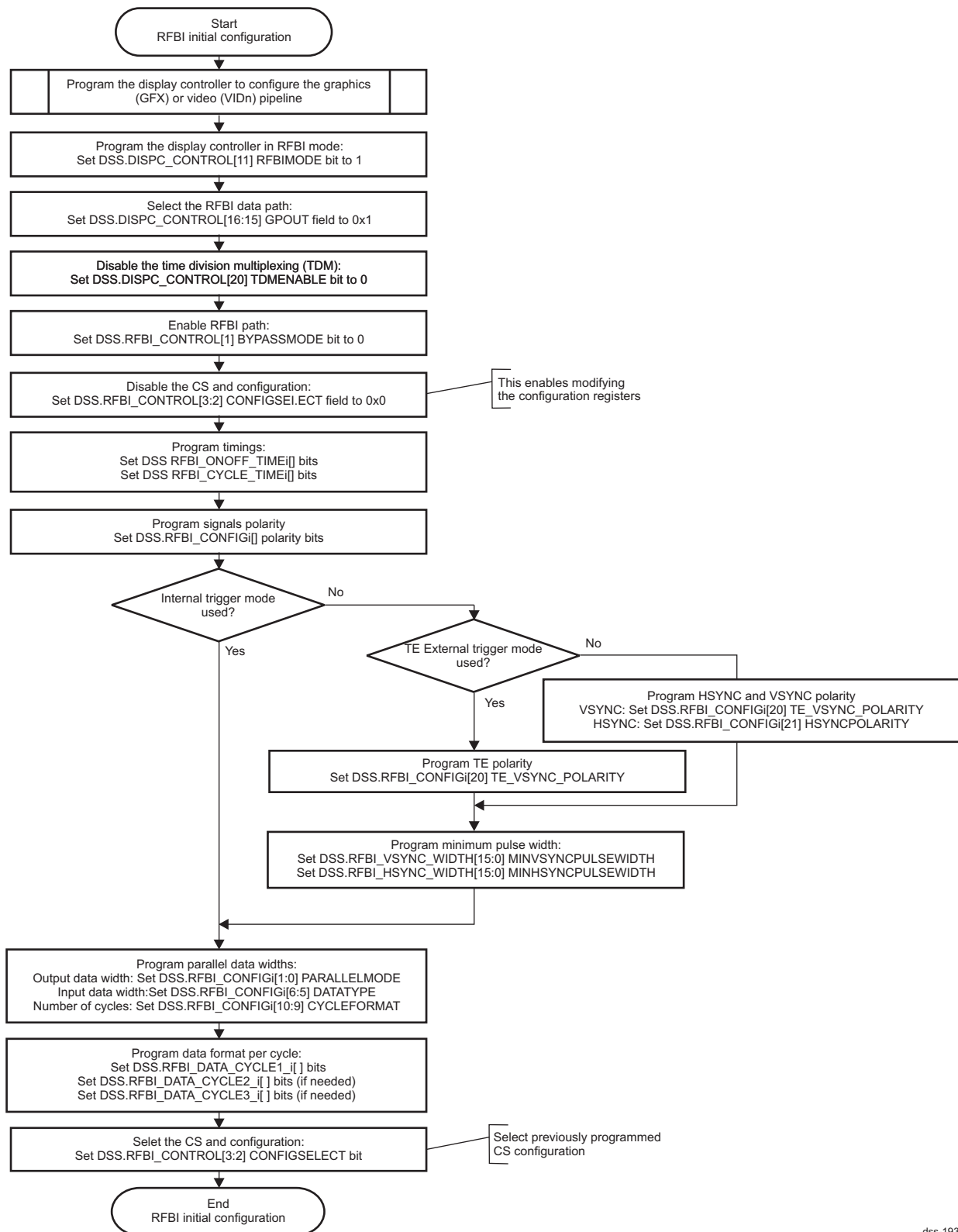
Figure 7-146 describes how to enable the RFBI module.
