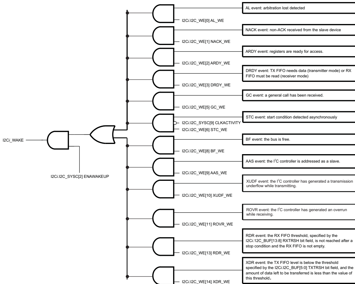
Figure 17-20. HS I 2 C Wake-up Generation Flow
