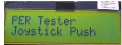
The transmitter is now configured for the PER test. The PER test is started by pushing the joystick (as a button). The transmitter will display the number of packets sent during the PER test. The PER test is stopped by pushing the joystick again.
