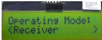
Select receiver on one of the SmartRF04EB's and transmitter on the other. Use the joystick to select mode. Confirm the selection by pressing Button S1.
