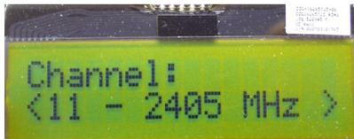
Select a channel between 11 and 26 (2405-2480 MHz). The channel is selected by navigating the joystick to the right or left. Confirm the selection by pressing Button S1.
