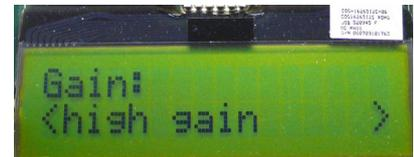
Select LNA gain on the CC2590 with the joystick. Either high gain or low gain mode are possible settings. Normally, high gain mode should be selected. Confirm the selection with Button S1. The receiver is now ready to receive packets.
