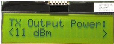
On the transmitter node, select the TX output power (signal strength). Use the joystick to select between -13 dBm, -3 dBm, 5 dBm, 10 dBm or 11 dBm. Confirm the selection with Button S1.
