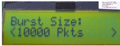
Select burst size (number of packets to send) by using the joystick, either 1000, 10K, 100K or 1M packets. Confirm the selection with Button S1.
