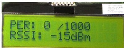
The PER test receiver will display the PER value (number of lost and erroneous packets divided by the total number of packets sent, displayed as a fraction of 1000). It will also display a moving average RSSI value (received signal strength). The test can be reset by pressing Button S1.
