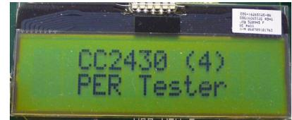
When power is applied to the SmartRF04EB, the preprogrammed PER test on the CC2430 will start running. The LCD will display the screen as shown in the picture above. The number in the parentheses is the revision of the CC2430. Press Button S1 to enter the menu.
