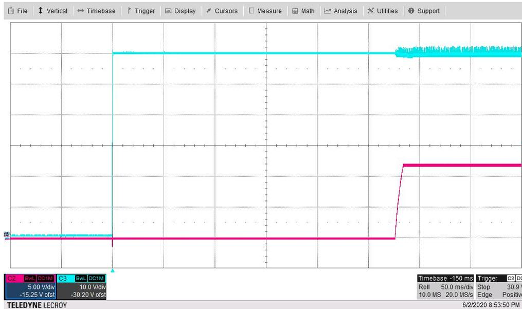
Figure 3-1. Output Voltage Start-up Waveform ( $V_{IN}$ : 10 V/div,  $V_{OUT}$ : 5 V/div, 50 ms/div)
