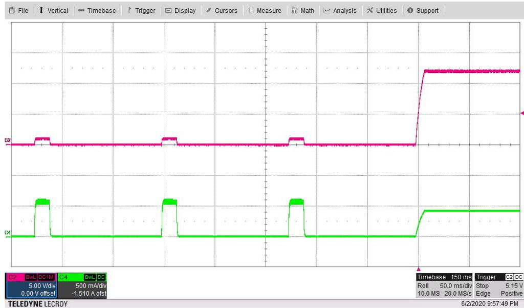
Figure 3-21. Short-Circuit Recovery ( $V_{OUT}$ : 5 V/div,  $I_{OUT}$ : 500 mA/div, 50 ms/div)
