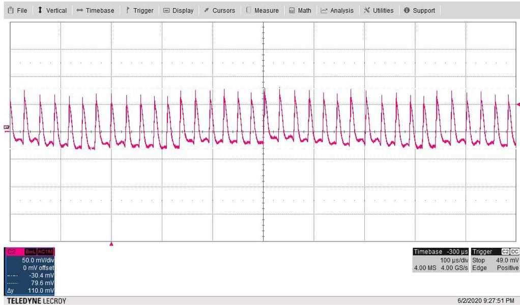
Figure 3-14. Output Voltage Ripple (AC Coupled) ( $V_{OUT}$ : 50 mV/div, 100 µs/div)
