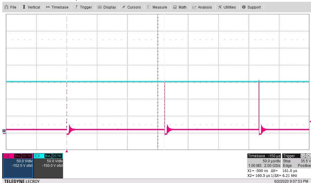
Figure 3-10. FET Switch Node Voltage (Vsnode: 50 V/div,  $V_{IN}$ : 50 V/div, 50  $\mu$ s/div)
