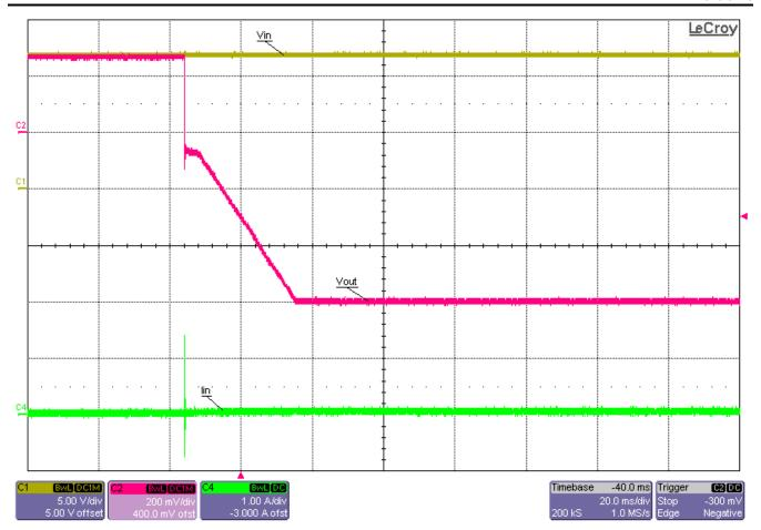
Figure 3-15. Start-up Into No Load, 12-V Input, -0.6-V Output, Start-up Initiated via the Enable Connection (Input Supply Already Turned ON)
