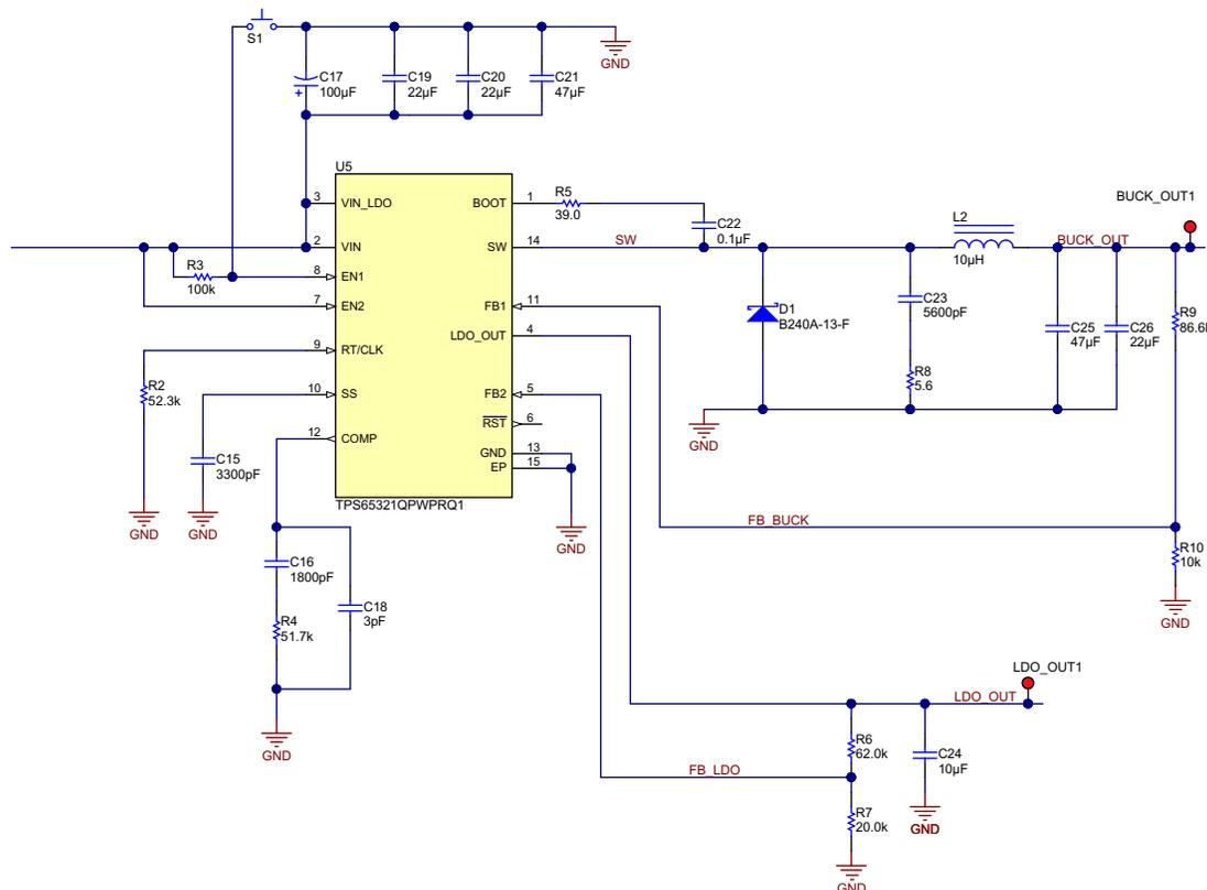
Figure 13. TPS65321-Q1 Current-Mode Buck Converter: 4.5- to 52-V Input
