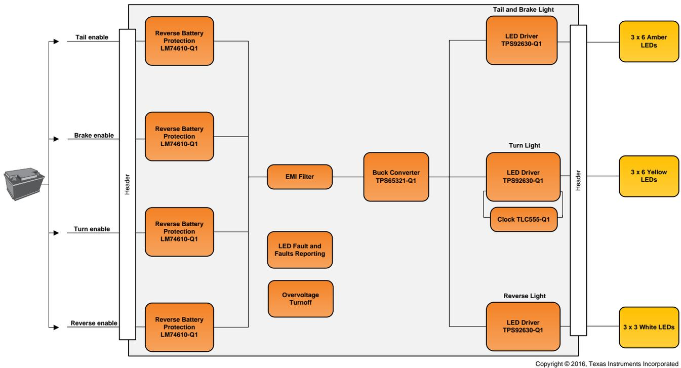
**Figure 1. Tail-Light System Driven From the Car Battery**
