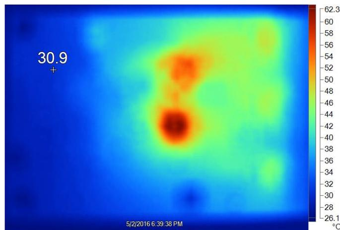
Figure 30. LM74610-Q1 Smart-Reverse Battery-Diode Temperature at 13.5-V Input Voltage
