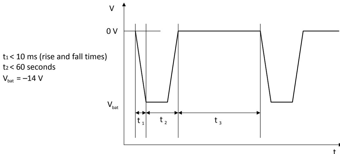
Figure 9. Reverse-Battery Pulse
