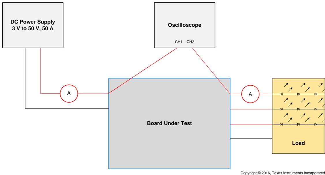
**Figure 27. Efficiency-Test Setup**
