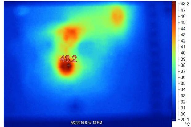
Figure 29. TPS65321-Q1 Buck-Converter Temperature Above 48.2°C at Three Strings of LEDs at 100 mA
