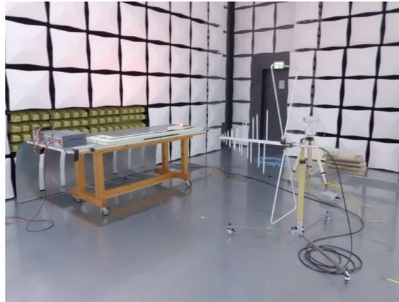
**Figure 43. Radiated Emissions Setup With a Logarithmic Antenna: 30 MHz to 2.5 GHz**
