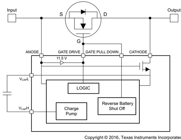
**Figure 5. LM74610-Q1 Zero  $I_Q$  Reverse-Polarity Protection Smart-Diode Controller**
