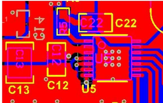
**Figure 51. Input and Output Capacitor Placement**
