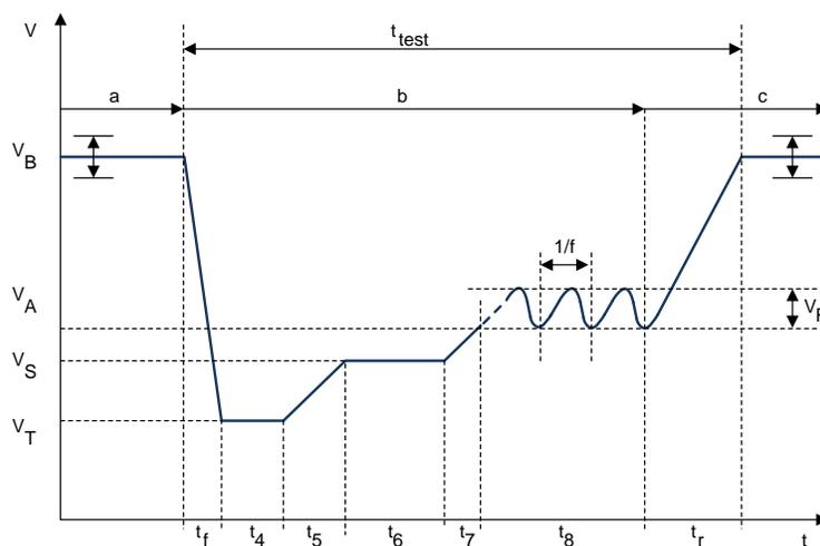
Figure 36. Cold-Crank Wave Shape
