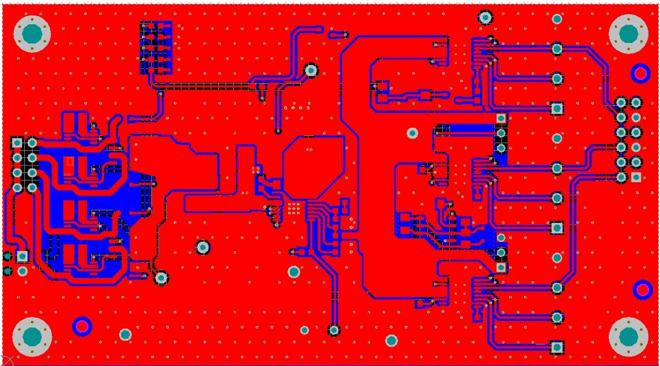
**Figure 52. Solid GND Fill**
