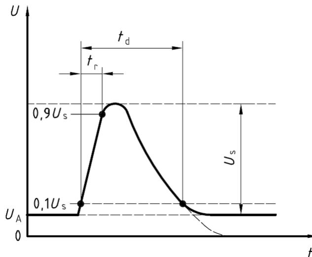
Figure 7. Load-Dump Pulse
