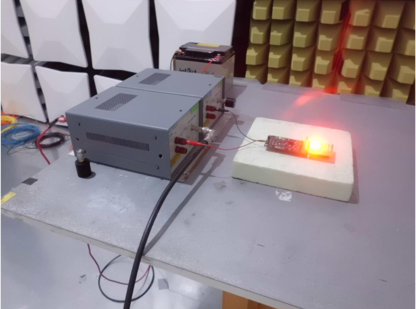
**Figure 38. Conducted-Emissions Setup**
