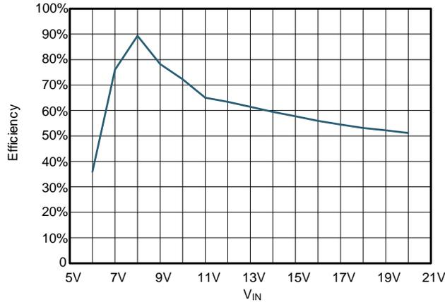
Figure 31. Efficiency Versus Input Voltage at  $I_{LED} = 100$  mA per String
