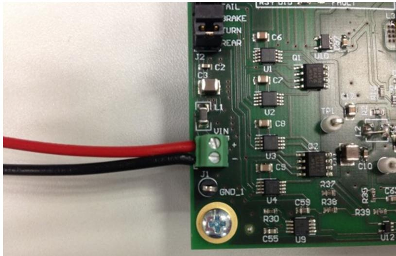
**Figure 22. Board Supply-Input Terminal**
