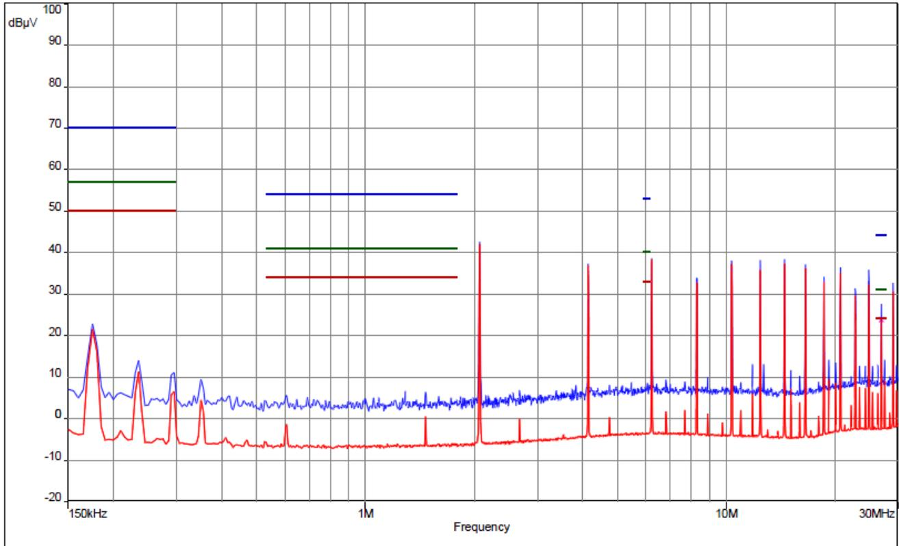
**Figure 41. Conducted Emissions: Line Side 150 kHz to 30 MHz**
