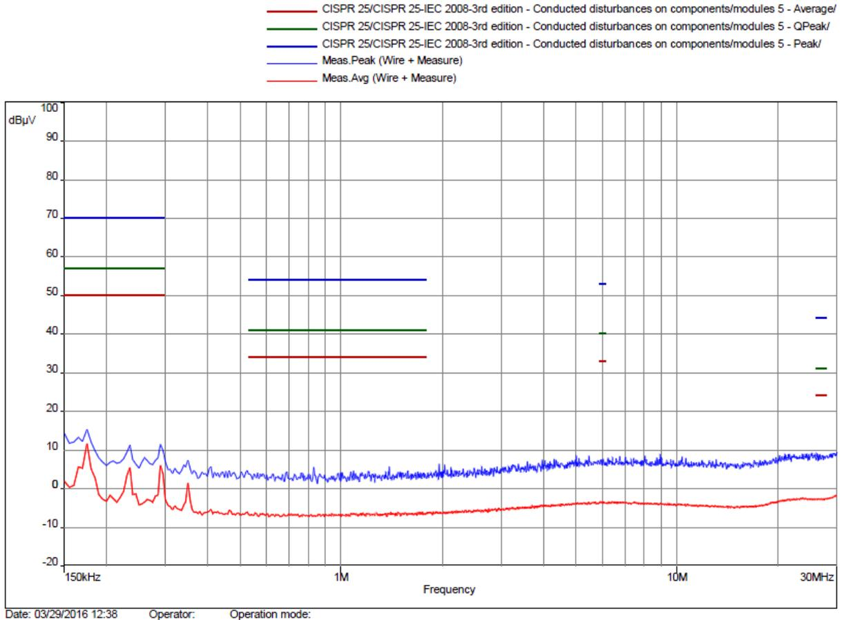
**Figure 39. Ambient-Noise Level: Line Side 150 kHz to 30 MHz**
