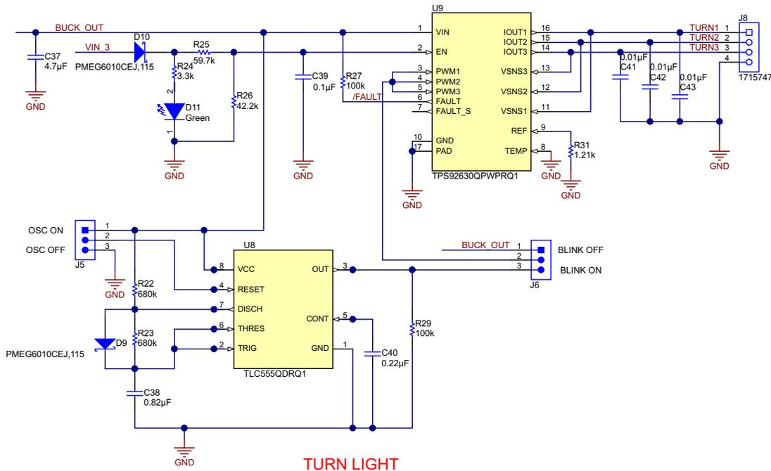
Figure 18. TPS92630-Q1 Three-Chanel LED Driver
