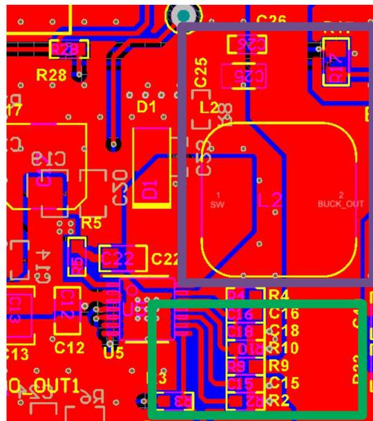
Figure 50. Routing of the Switching Converter
