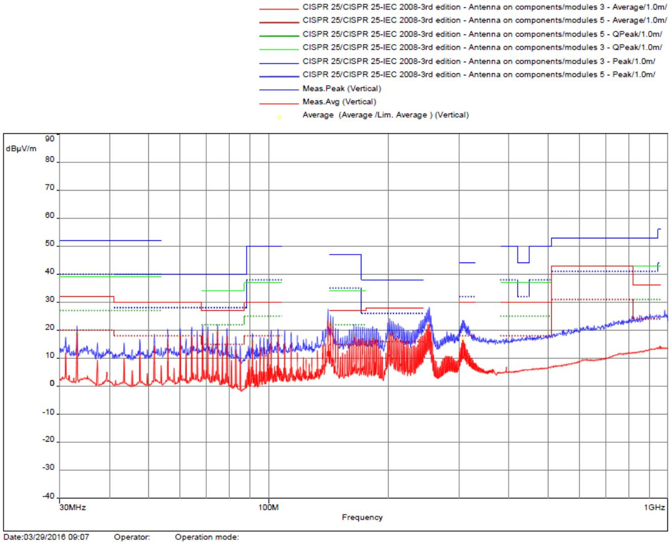
**Figure 46. Radiated Emissions: Line Side 30 MHz to 1 GHz**
