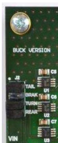
**Figure 20. Jumper J2 for Setting the Type of Light**
