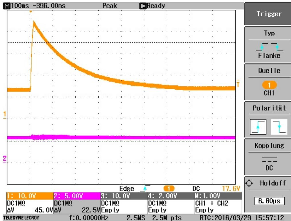
Figure 33. Load Dump and Output: No Turnoff
