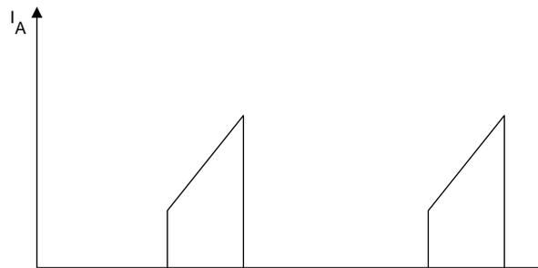
**Figure 15. Input-Current Waveform**
