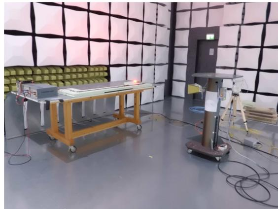
**Figure 44. Radiated Emissions Setup With a Horn Antenna: 1.447 GHz to 1 GHz**
