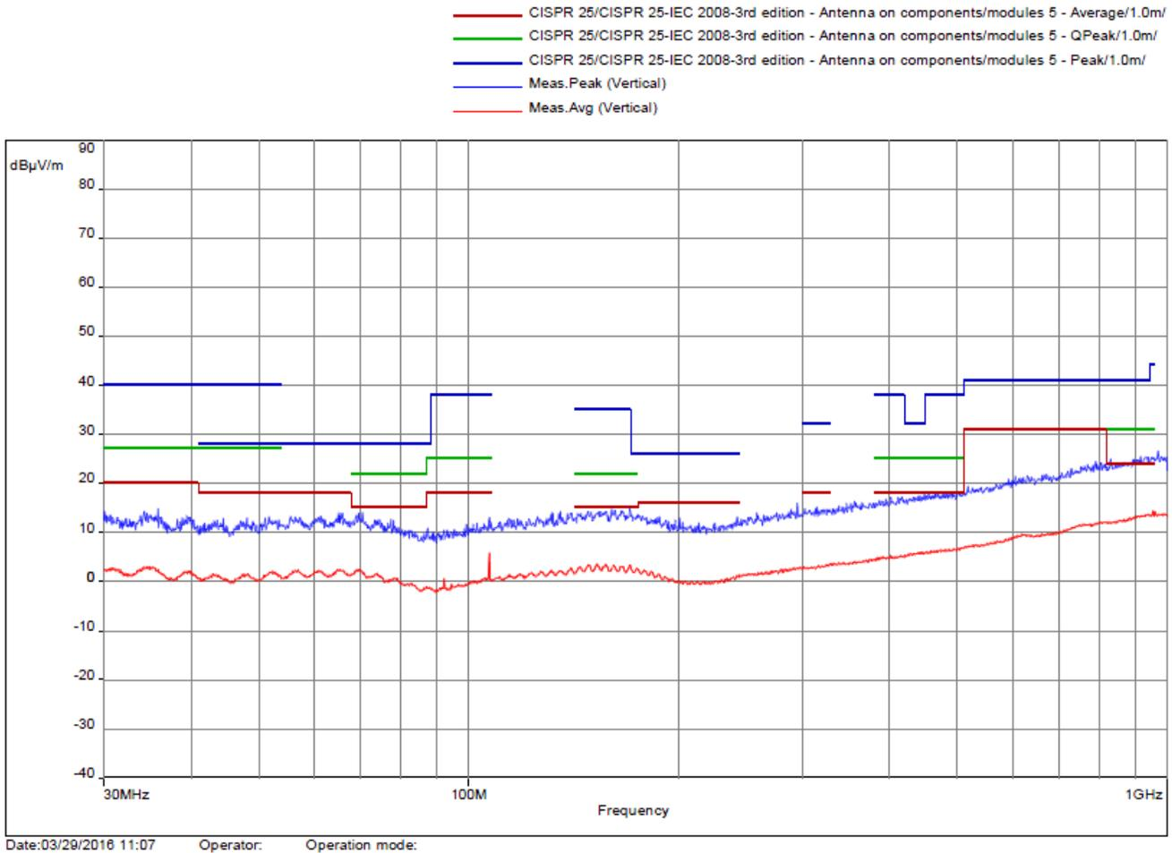
Figure 45. Ambient-Noise Level of Radiated Emissions: Line Side 30 MHz to 1 GHz
