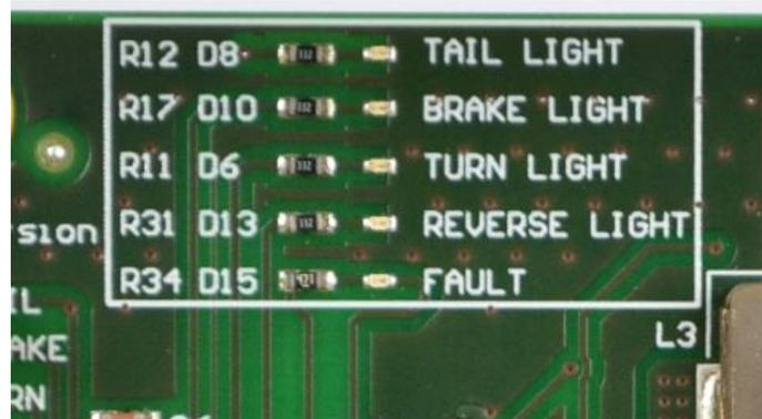
**Figure 23. LEDs Indicating Failures and On Lights**
