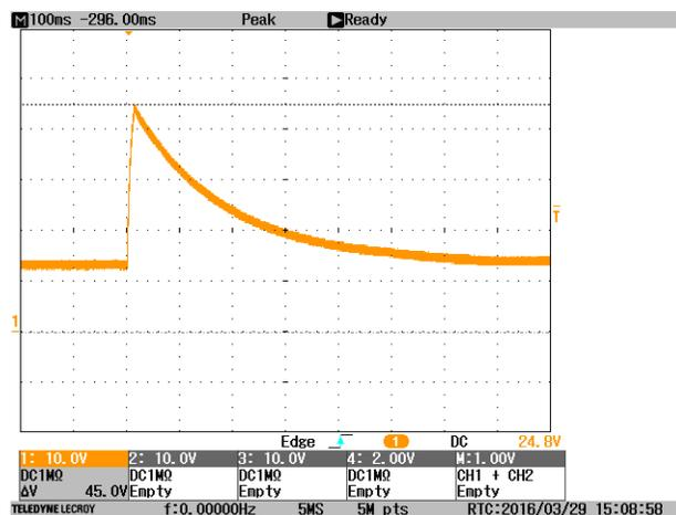
Figure 32. ISO 7637-2:2004 Pulse 4 Load Dump
