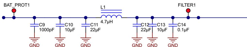
**Figure 14. Input-Voltage Noise Filter**
