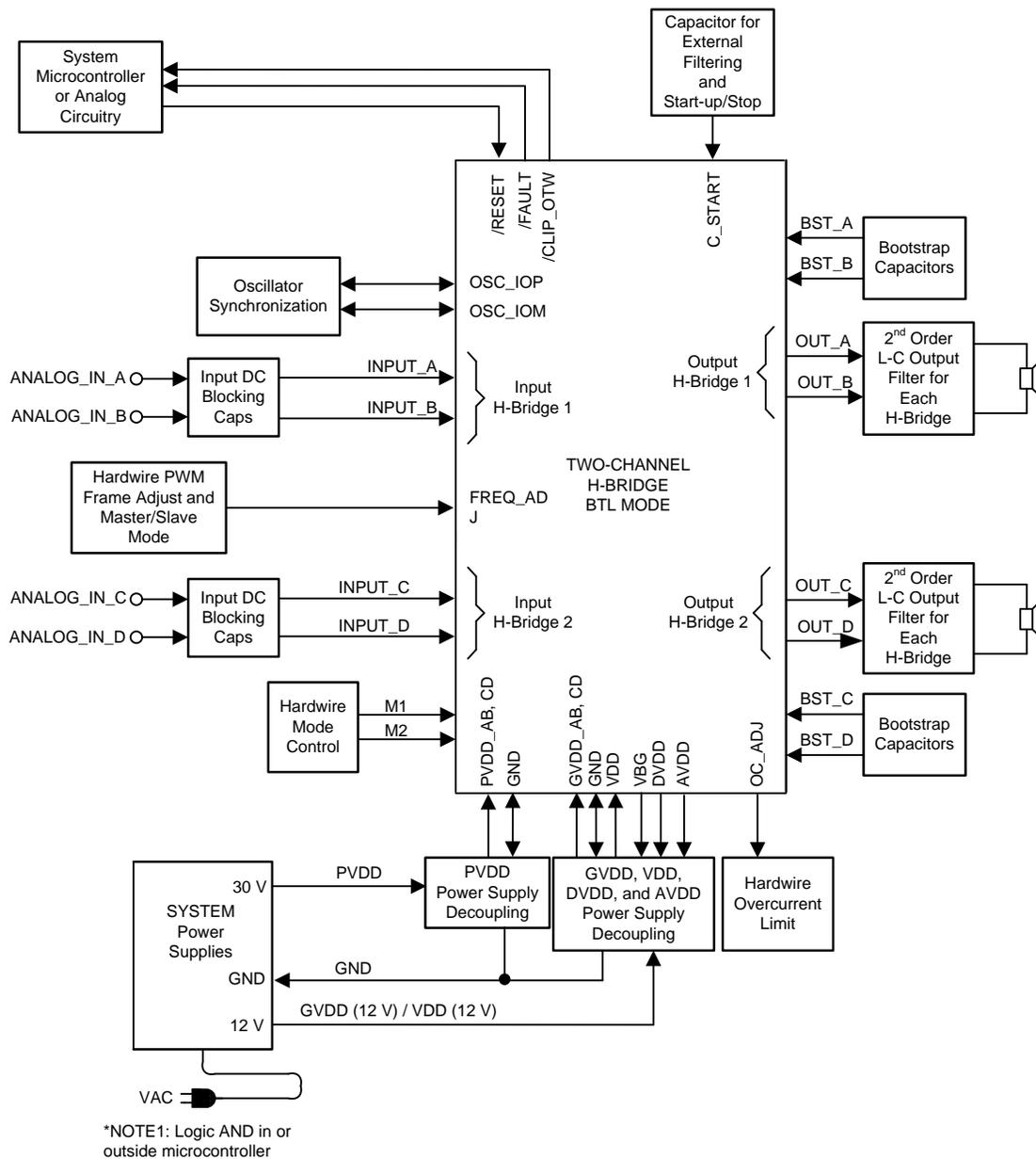
Figure 2. TPA3244 Block Diagram
