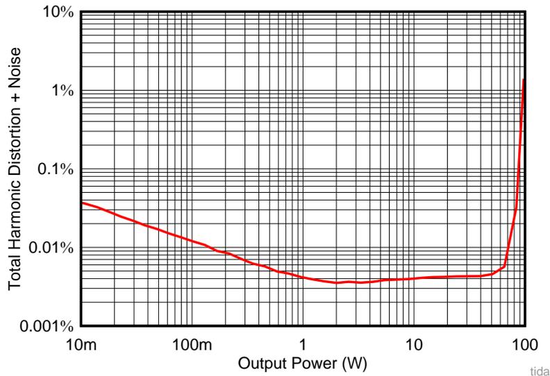
Figure 17. Total Harmonic Distortion + Noise versus Power
