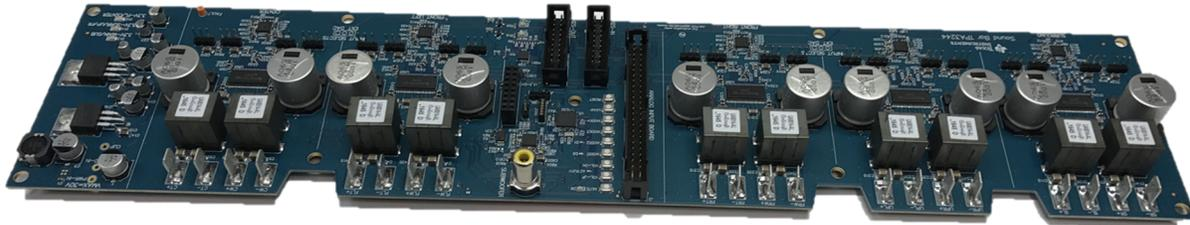
**Figure 5. Amplifier and DAC PCB**
