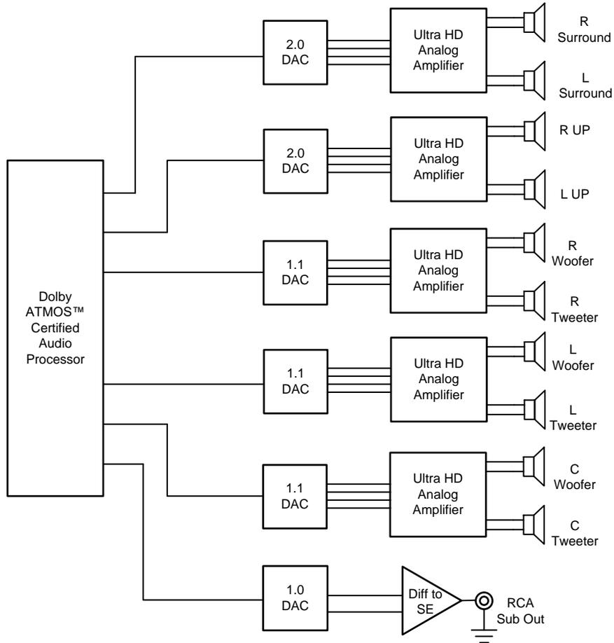
Figure 1. TIDA-01414 Block Diagram
