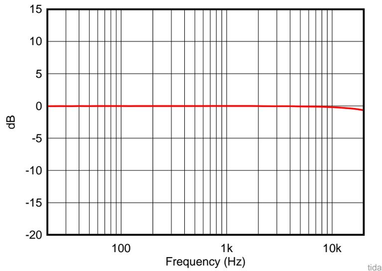
Figure 15. Soundbar Frequency Response
