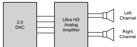
**Figure 7. Amplifier and DAC in 2.0 Configuration (Surround Left, Surround Right, Up-Firing Left and Up-Firing Right on Soundbar)**
