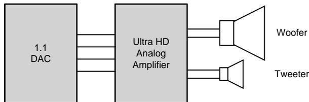
**Figure 6. Amplifier and DAC in 1.1 Configuration (Left, Center, and Right Channels on Soundbar)**
