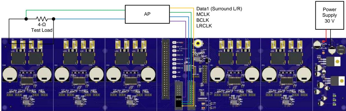
Figure 14. Soundbar Test Setup
