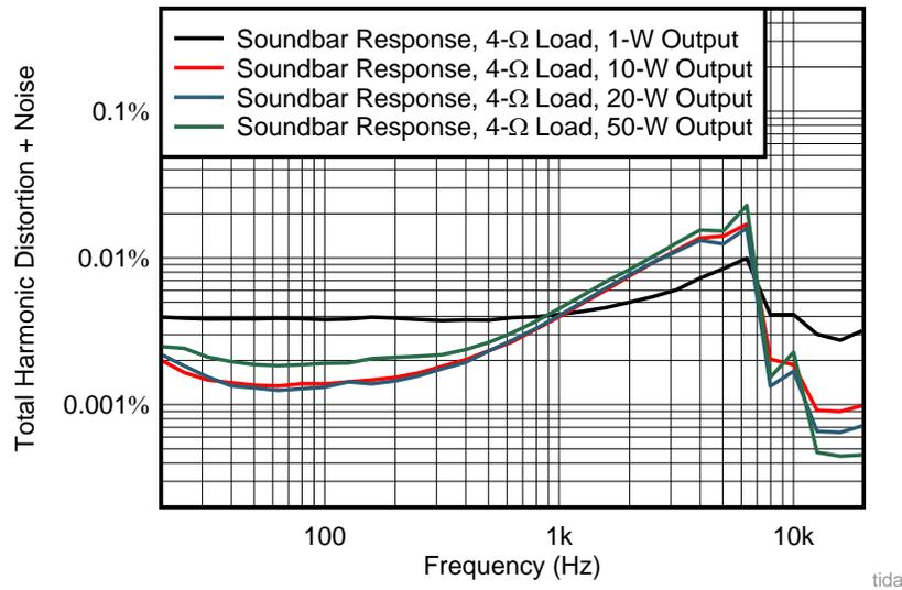
Figure 16. Total Harmonic Distortion + Noise versus Frequency
