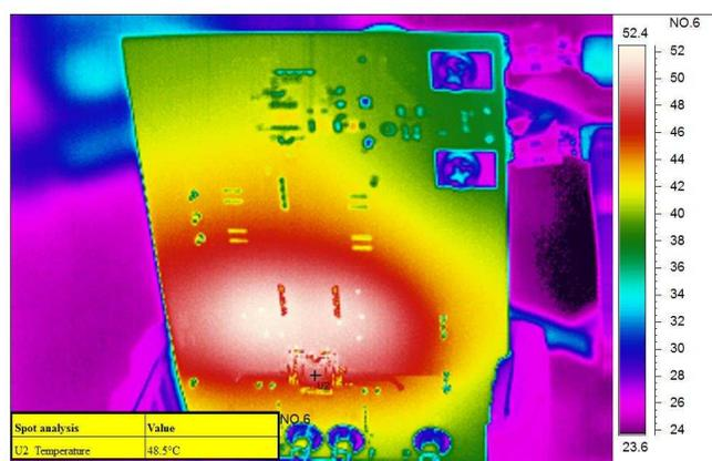
Figure 27. Thermal Measurement at 14-V Input (Back)
