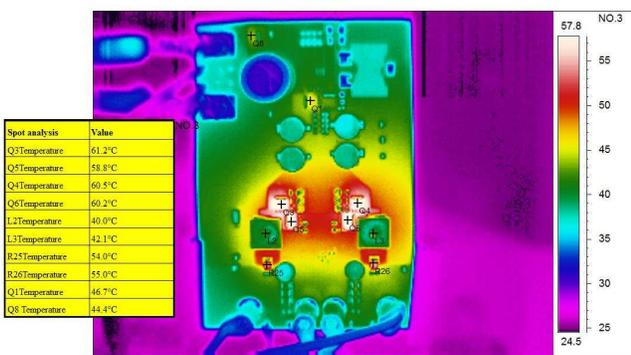
Figure 24. Thermal Measurements at 11-V Input (Front)
