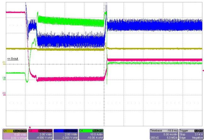
Figure 10. 5-V Output During Crank Test Pulse (Zoomed)
