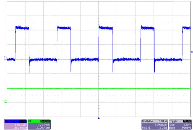
**Figure 17. 3.3-V Output Switch Node**
