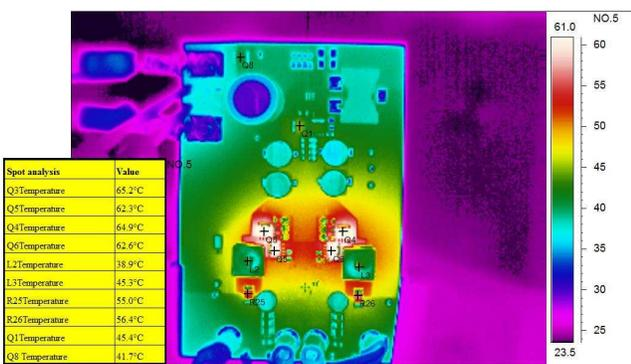
Figure 26. Thermal Measurements at 14-V Input (Front)
