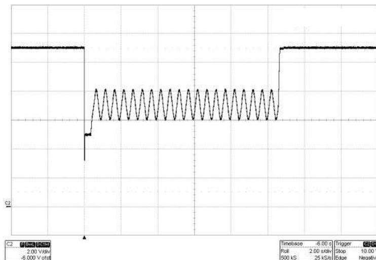
**Figure 6. Program 3, 2 s/div—Volkswagen Cold-Start Test Pulse, VW 80000**
