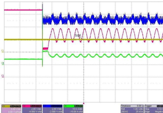
Figure 9. 5-V Output During Crank Test Pulse
