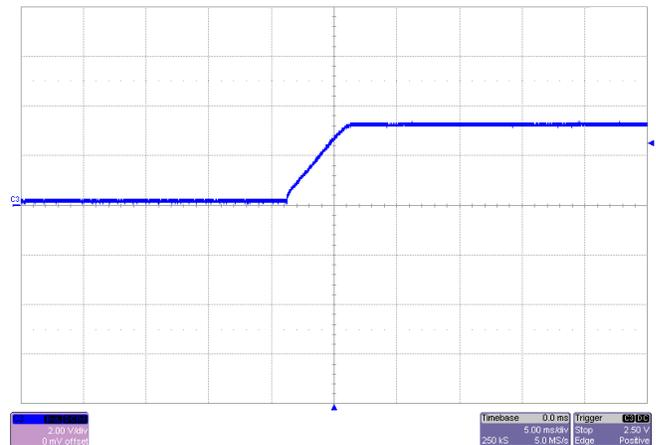
Figure 13. 3.3-V Output Start-Up (No Load)
