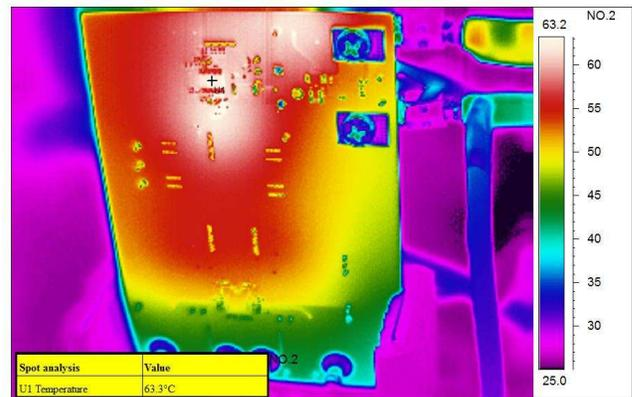
Figure 23. Thermal Measurement at 6-V Input (Back)
