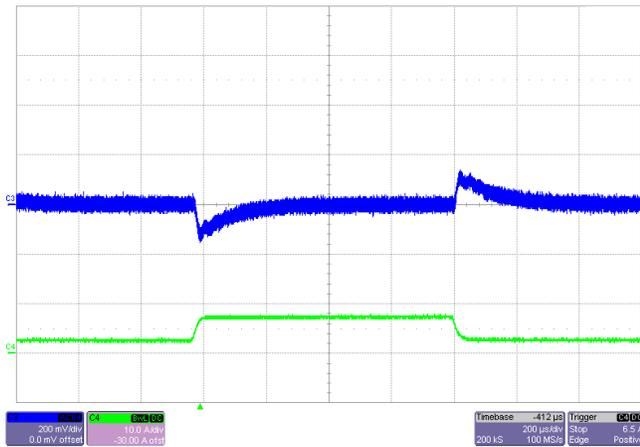
**Figure 18. 5-V Output Load Transient Response**
