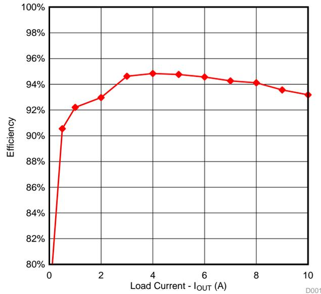
Figure 20. 5-V Output Efficiency
