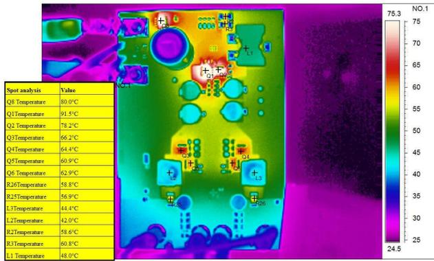
Figure 22. Thermal Measurements at 6-V Input (Front)
