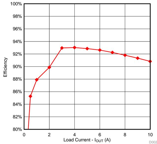
**Figure 21. 3.3-V Output Efficiency**
