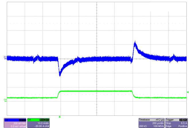
**Figure 19. 3.3-V Output Load Transient Response**
