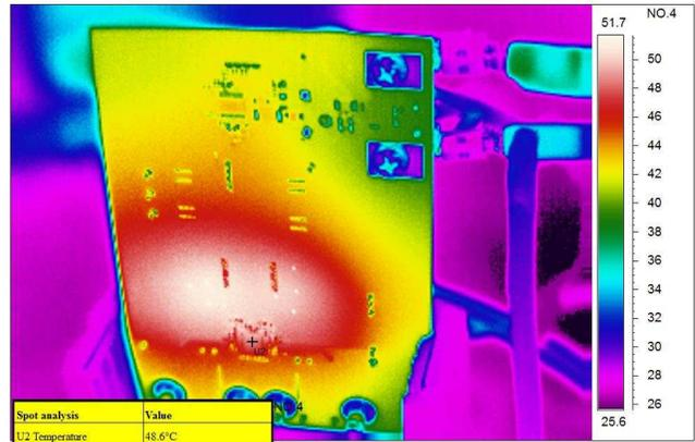
Figure 25. Thermal Measurement at 11-V Input (Back)
