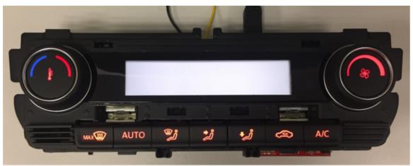
This TI design uses TPS7B4250-Q1 (tracking LDO) and SN74LV4051-Q1 (multiplexer, demultiplexer) to drive and multiplex the eight off board temperature (NTC) sensors.
