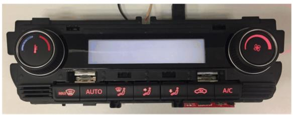
Figure 32. LED Dimming With 100% Duty Cycle
