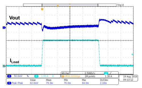
Figure 3-4. Vin = 3.3V, Vout = 2.5 V, ILoad 10mA to 3A and Vpp ~  $\pm$ 42mV
