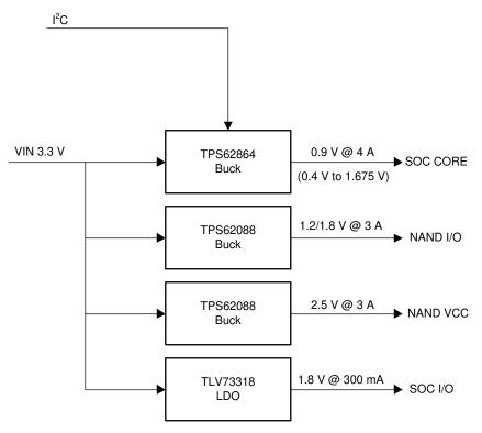
Figure 2-1. TIDA-050044 Block Diagram
