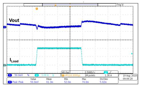
Figure 3-3. Vin = 3.3V, Vout = 1.2 V, ILoad 10mA to 2A and Vpp ~ ±37mV
