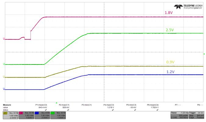
Figure 3-1. Startup with no Load
