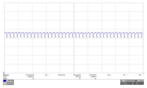
Figure 3-7. Vin = 3.3 V, Vout = 2.5 V, ILoad = 1.7A and Vpp ~13.0mV
