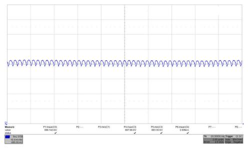
Figure 3-5. Vin = 3.3 V, Vout = 0.9V, ILoad = 2.0A and Vpp ~ 5mV
