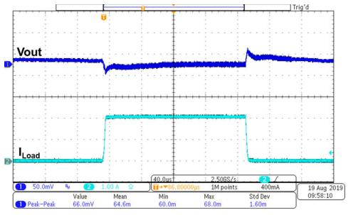
Figure 3-2. Vin = 3.3 V, Vout = 0.9 V, ILoad 5mA to 2A and Vpp ~ ±35mV
