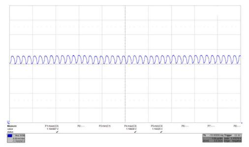
Figure 3-6. Vin = 3.3 V, Vout = 1.2 V, ILoad = 1.2A and Vpp ~ 3mV
