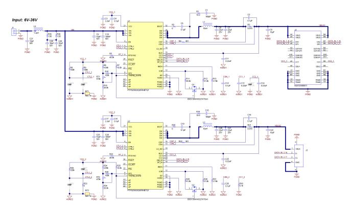
Figure 7. Type A And Type-C Dual Port Application Schematic
