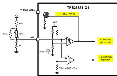
Figure 9. NTC Input Pin
