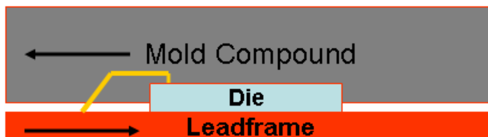
Figure 4. Cross Section Showing Mold Compound to Die Pad Delamination
