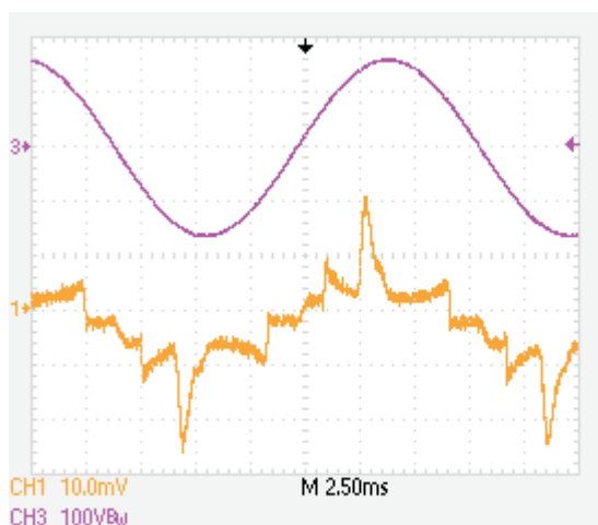
Figure 9. Input AC Voltage and Current, Full Load, No Dimmer (CH1 = I_{IN} , CH3 = V_{IN} (115 VAC), scale = 100 mA/div)
