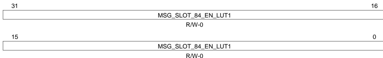
Figure 122. Protocol Encoder 84 Count Message Enable Bits [63-32] (PE_LINK_84_EN_LUT1_CFG) register
