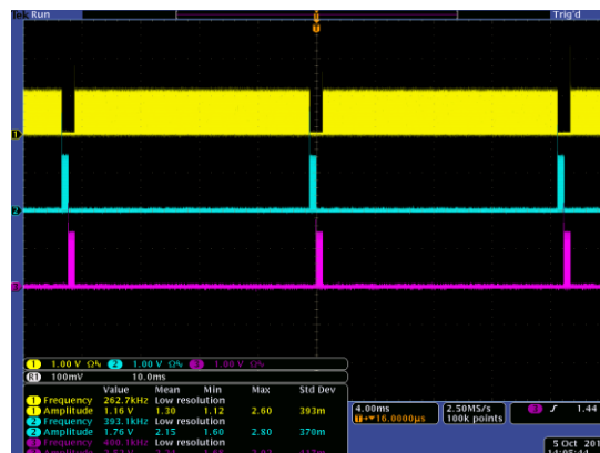
Figure 19: Sensor multiplexing – proximity (yellow), cap touch button 1 & 2 (green, magenta)
