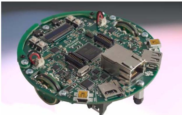
The Stellaris® LM3S9B92 EVALBOT Robotic Evaluation Board (EVALBOT) is a robotic evaluation platform for the Stellaris LM3S9B92 microcontroller. The board also uses a range of Texas Instruments' analog components for motor drive, power supply, and communications functions. After a few minutes of assembly, the EVALBOT's electronics are ready-to-run.
