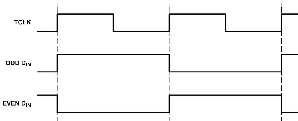
**Figure 2. Worst-Case Serializer I<sub>CC</sub> Test Pattern**
