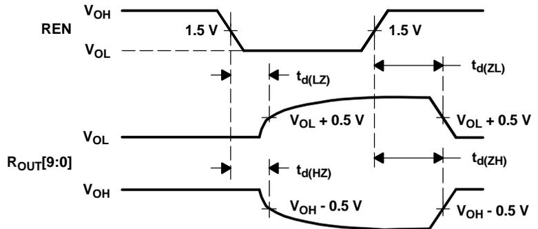
Figure 15. Deserializer High-Impedance-State Test Circuit and Timing
