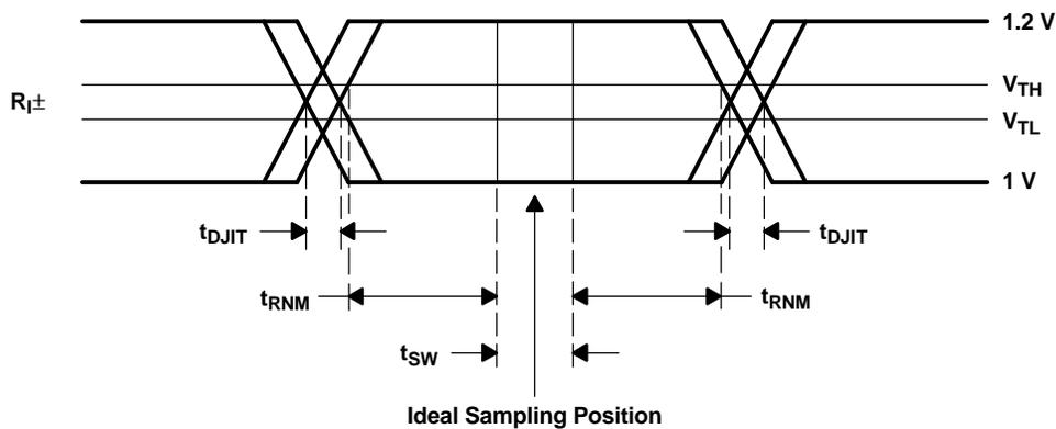
$t_{sw}$ : Setup and Hold Time (Internal Data Sampling Window)
