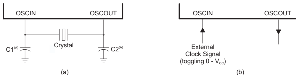
Figure 8. Crystal/Clock Connection
