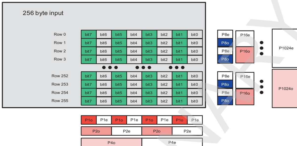
Figure 15-82. ECC Computation for a 256-Byte Data Stream (Read or Write)
