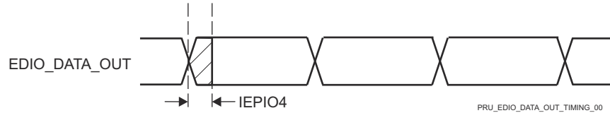
图 7-100. PRU_ICSSG IEP Digital IOs Timing Requirements
