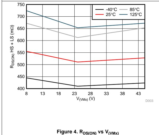
Figure 4.  $R_{DS(ON)}$  vs  $V_{VMx}$
