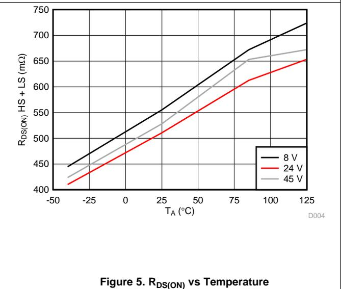
Figure 5.  $R_{DS(ON)}$  vs Temperature
