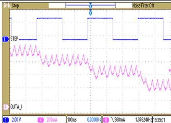
**Figure 10. Microstepping Current (Phase A) vs STEP Input, Mixed Decay on Decreasing Steps**
