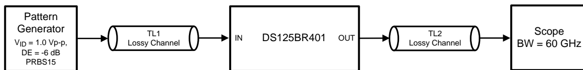
Figure 10. Test Setup Connections Diagram
