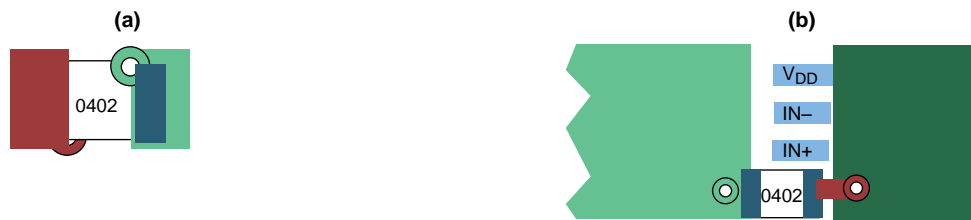
图 18. Typical Decoupling Capacitor Layouts
