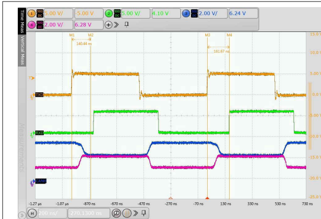
图 8-15. Typical TXD, RXD, CANH and CANL Waveforms at 2 Mbps
