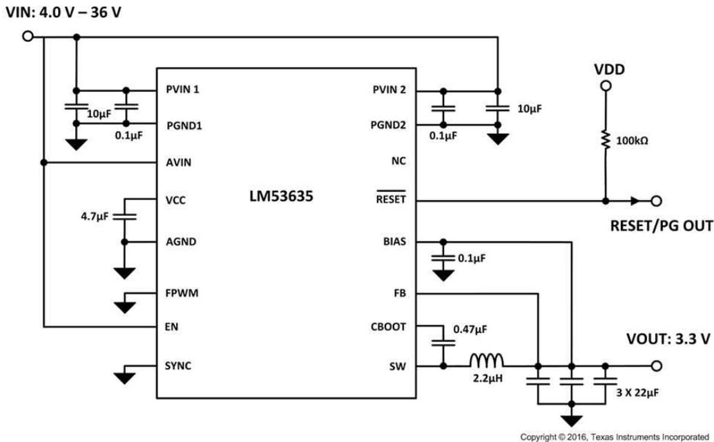
**图 9-18. Fixed 3.3-V, 3.5-A Output Power Supply**
