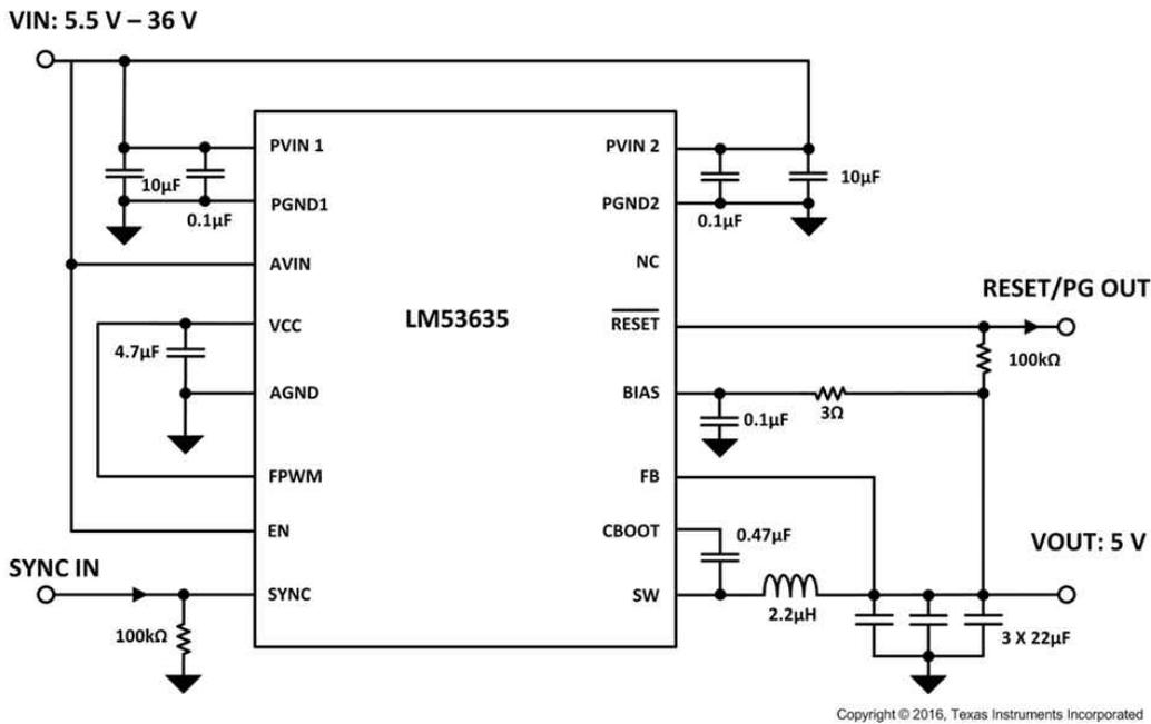
**图 9-4. Fixed 5-V, 3.5-A Output Power Supply**
