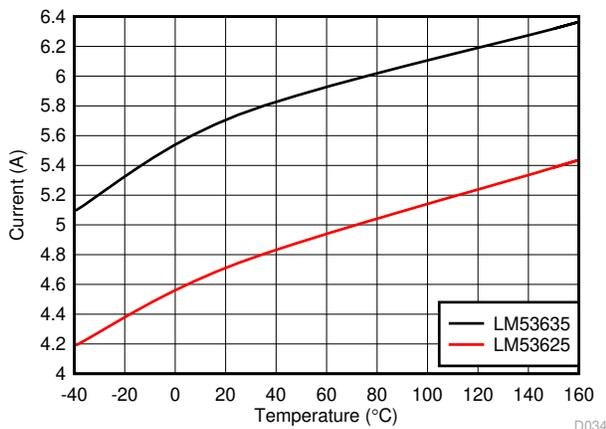
图 7-3. High Side/Peak Current Limit for LM53625/35-Q1
