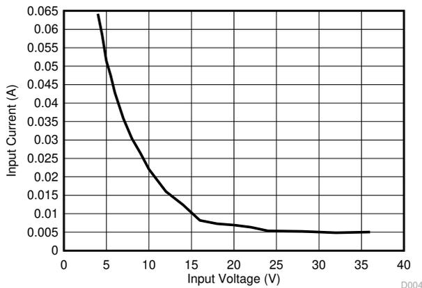
图 7-5. Short Circuit Average Input Current for LM53635-Q1
