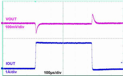
FPWM  $V_{OUT} = 3.3\text{ V}$   $L = 2.2\ \mu\text{H}$ ,
