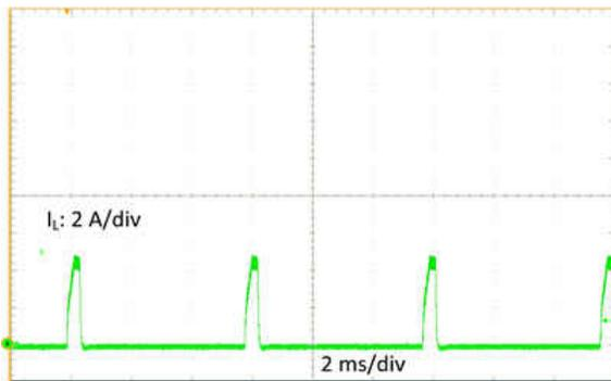
图 8-5. Inductor Current Bursts in Short Circuit
