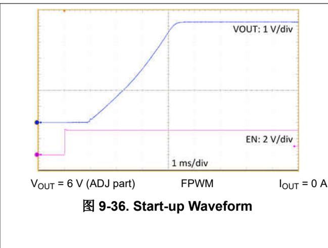
**图 9-36. Start-up Waveform**
