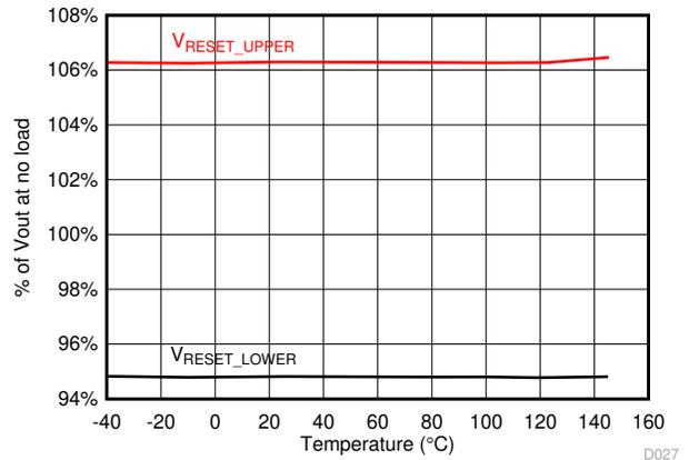
图 7-8. RESET Threshold as Percentage of Output Voltage
