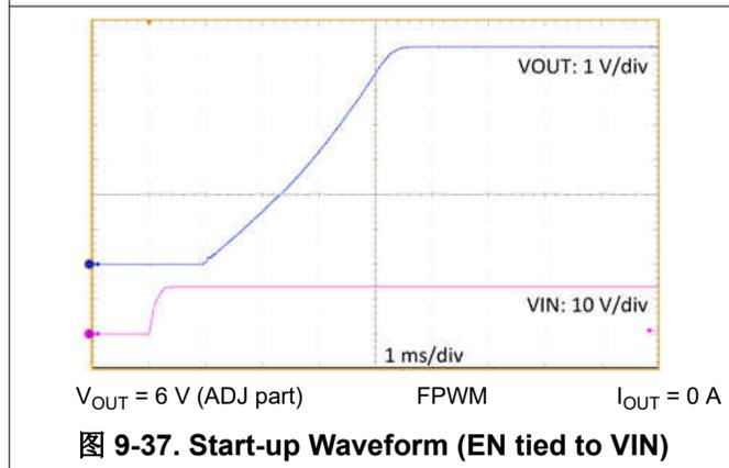
**图 9-37. Start-up Waveform (EN tied to VIN)**
