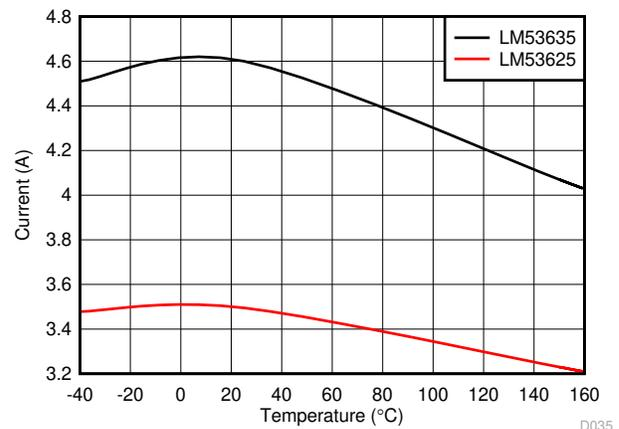
图 7-4. Low Side/Valley Current Limit for LM53625/35-Q1
