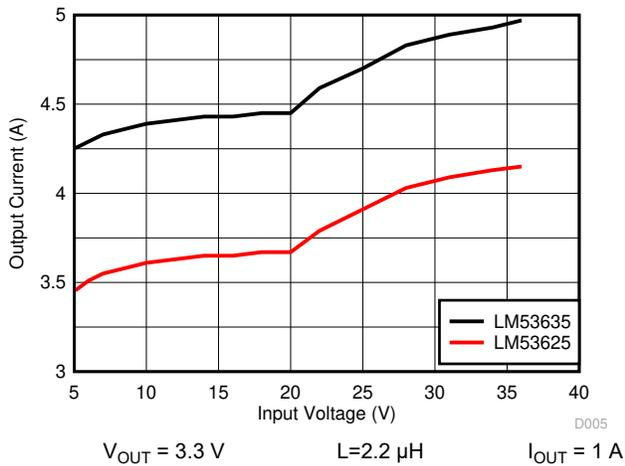
图 9-29. Output Current Level for Overcurrent Protection Trip
