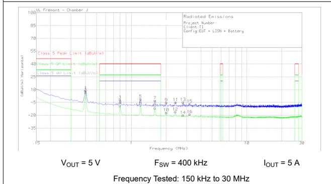
图 9-27. Radiated EMI Rod versus CISPR25 Limits
