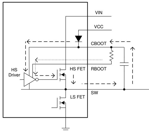
图 8-14. Simplified Circuit Showing How RBOOT Functions
