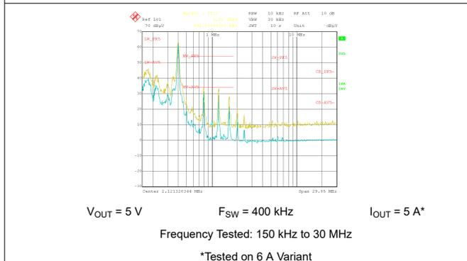
图 9-25. Conducted EMI versus CISPR25 Limits (Yellow: Peak Signal, Blue: Average Signal)
