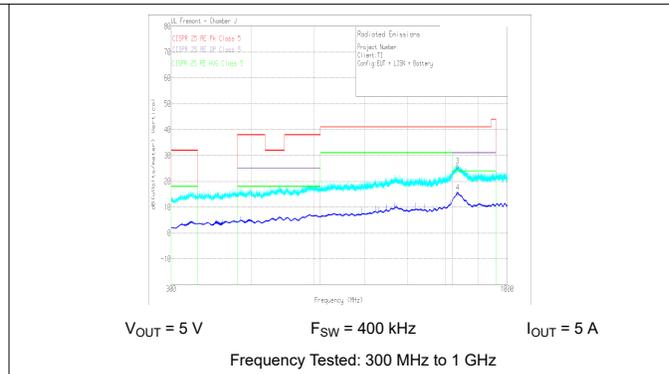
图 9-30. Radiated EMI Log Vertical versus CISPR25 Limits
