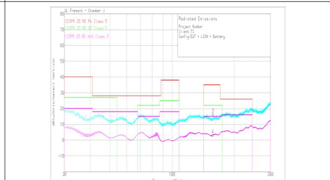
图 9-28. Radiated EMI Bicon Vertical versus CISPR25 Limits
