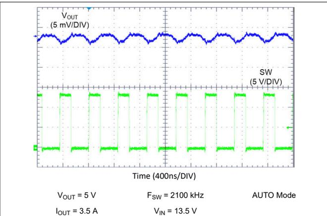
图 9-18. LM62435-Q1 Switching Waveform and  $V_{OUT}$  Ripple
