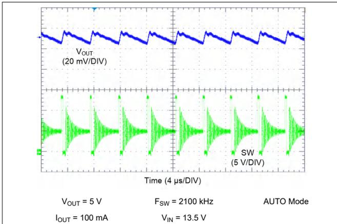
图 9-17. LM62435-Q1 Switching Waveform and  $V_{OUT}$  Ripple
