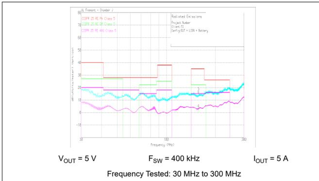
图 9-29. Radiated EMI Bicon Horizontal versus CISPR25 Limits
