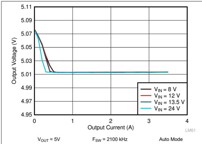
图 9-11. LM62435-Q1 Load and Line Regulation
