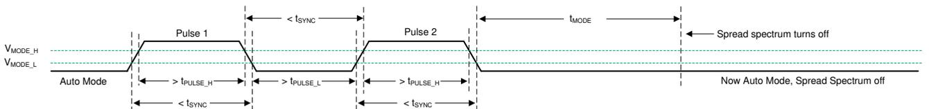
图 8-7. Spread Spectrum Disabled in Auto Mode
