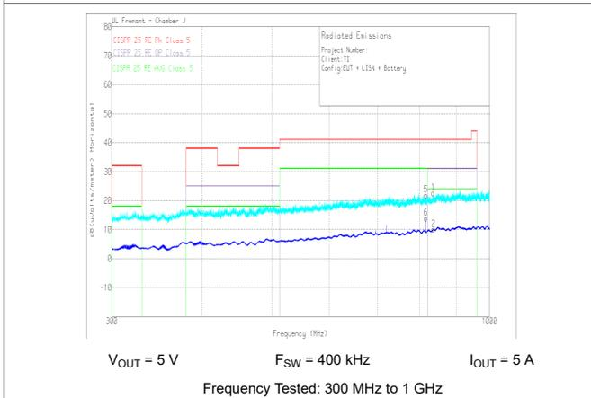
图 9-31. Radiated EMI Log Horizontal versus CISPR25 Limits
