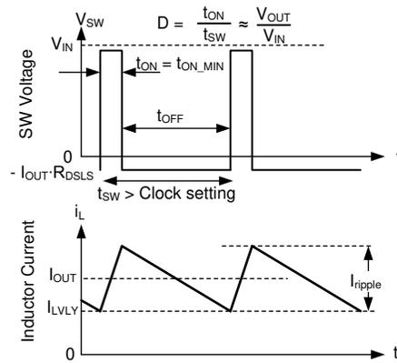
In valley control mode, minimum inductor current is regulated, not peak inductor current.
