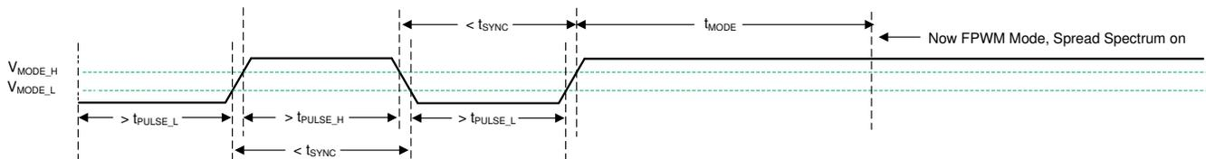
图 8-11. Transition from SYNC Mode to FPWM Mode
