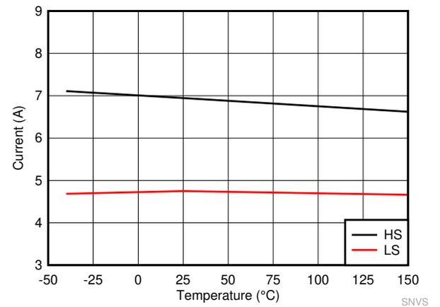
图 7-4. LM62435-Q1 High-side and Low-side Current Limits
