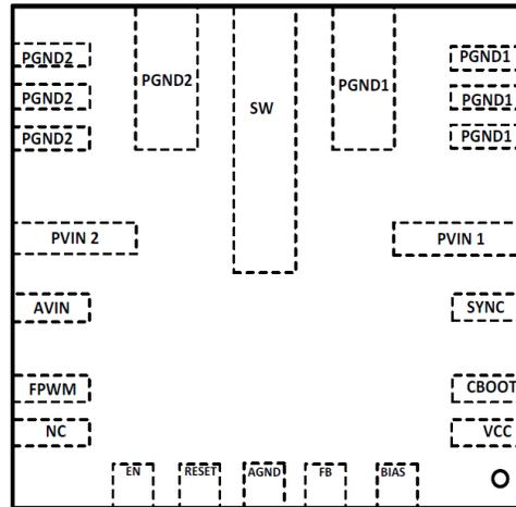
图 6-1. RNL Package 22-Pin VQFN Top View
