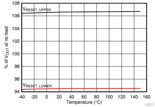
图 7-8. RESET Threshold as Percentage of Output Voltage
