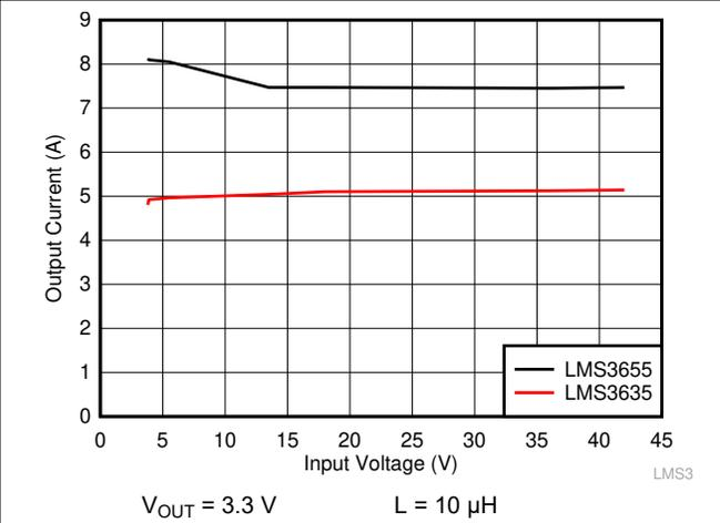
图 9-26. Output Current Level for Overcurrent Protection Trip
