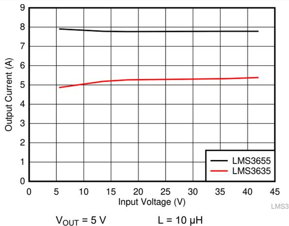
图 9-13. Output Current Level Limit Before Overcurrent Protection
