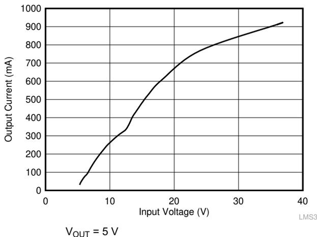
图 9-9. Load Current for PFM-to-PWM Transition
