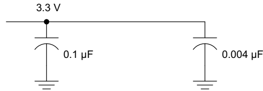
图 9-2. Recommended M-LVDS Bypass Capacitor Layout
