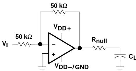
**Figure 60. Series-Resistance Circuit**
