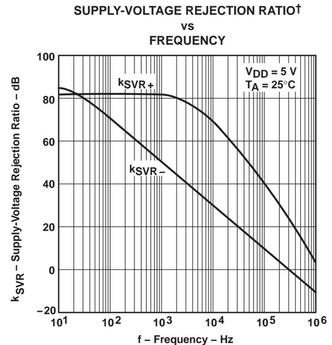
† For all curves where  $V_{DD} = 5\text{ V}$ , all loads are referenced to 2.5 V. For all curves where  $V_{DD} = 3\text{ V}$ , all loads are referenced to 1.5 V.
