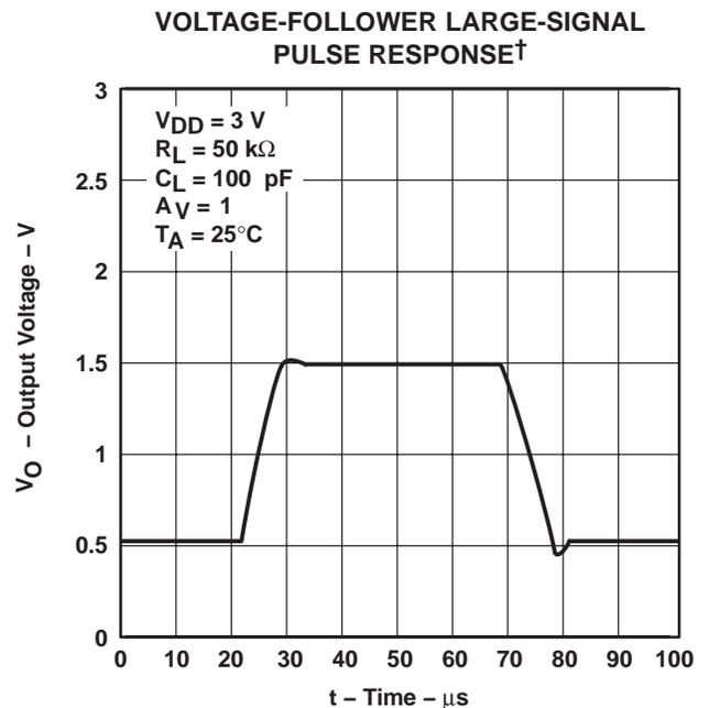
† Data at high and low temperatures are applicable only within the rated operating free-air temperature ranges of the various devices.
