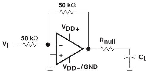
**Figure 60. Series-Resistance Circuit**
