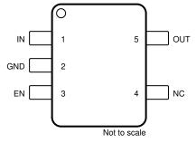
图 5-2. DBV Package, 5-Pin SOT-23, Top View
