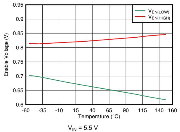
图 6-12. EN High and Low Threshold vs Temperature
