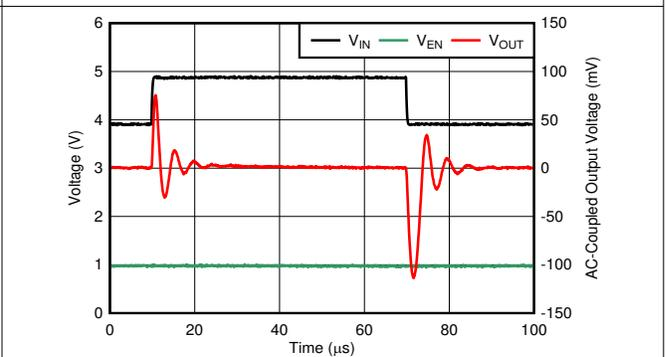
$V_{IN} = 3.9\text{ V}$  to  $4.9\text{ V}$ , slew rate =  $1\text{ V}/\mu\text{s}$ ,  $V_{EN} = 1\text{ V}$ ,  $I_{OUT} = 300\text{ mA}$
