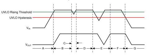
图 7-2. Typical UVLO Operation
