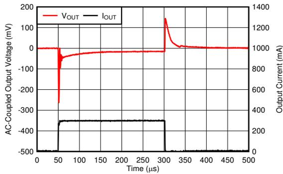
$V_{IN} = 3.9\text{ V}$ ,  $V_{EN} = 1\text{ V}$ ,  $I_{OUT} = 1\text{ mA}$  to  $300\text{ mA}$ ,
