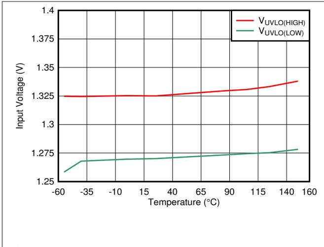
图 6-13. UVLO Rising and Falling Threshold vs Temperature
