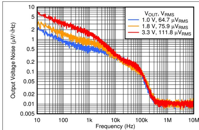
图 6-17. Output Noise vs Frequency and  $V_{OUT}$
