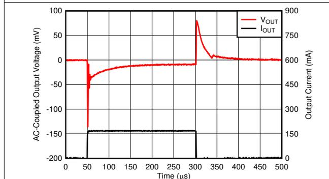
$V_{IN} = 3.9\text{ V}$ ,  $V_{EN} = 1\text{ V}$ ,  $I_{OUT} = 1\text{ mA}$  to  $150\text{ mA}$ , slew rate =  $1\text{ A}/\mu\text{s}$
