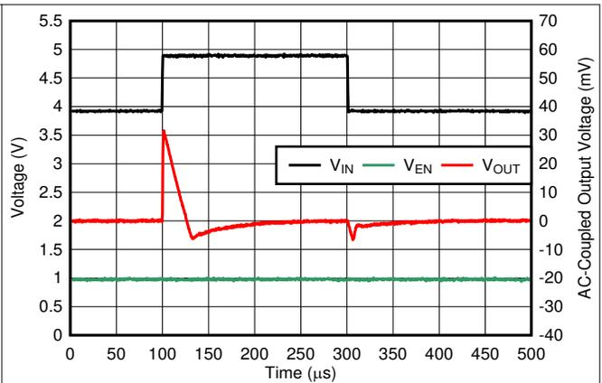
$V_{IN} = 3.9\text{ V}$  to  $4.9\text{ V}$ , slew rate =  $1\text{ V}/\mu\text{s}$ ,  $V_{EN} = 1\text{ V}$ ,  $I_{OUT} = 1\text{ mA}$
