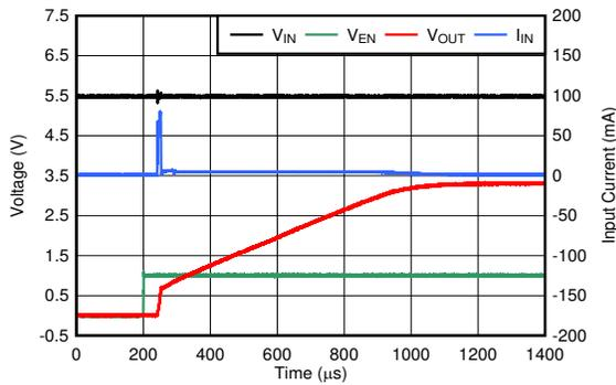
$V_{IN} = 5.5\text{ V}$ ,  $C_{IN} = \text{open}$ ,  $I_{OUT} = \text{open}$
