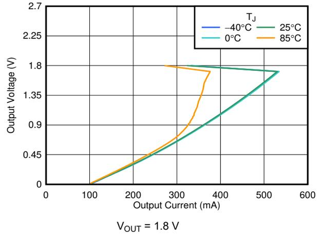
图 6-8. Foldback Current Limit vs  $I_{OUT}$
