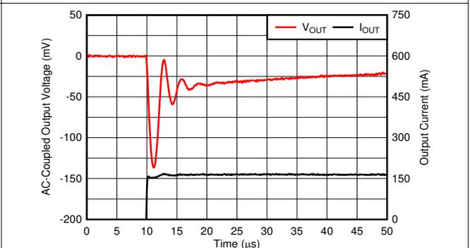
$V_{IN} = 3.9\text{ V}$ ,  $V_{EN} = 1\text{ V}$ ,  $I_{OUT} = 1\text{ mA}$  to  $150\text{ mA}$ , slew rate =  $1\text{ A}/\mu\text{s}$ , rising edge
