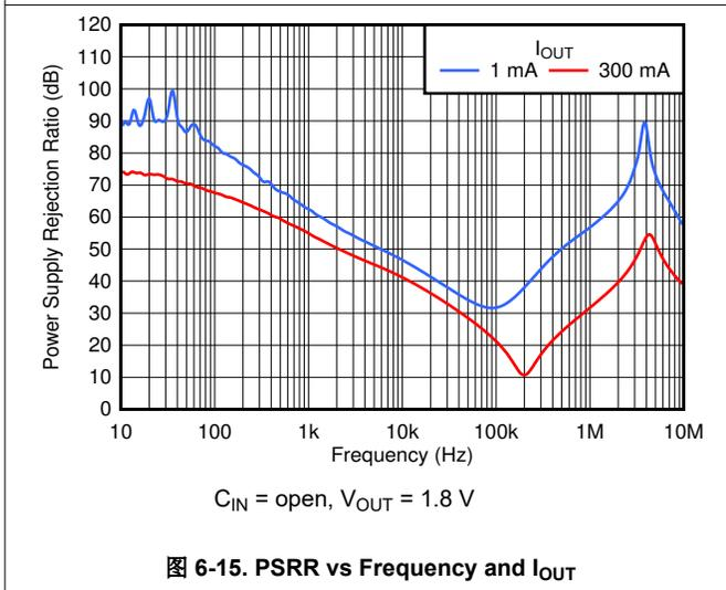
图 6-15. PSRR vs Frequency and  $I_{OUT}$
