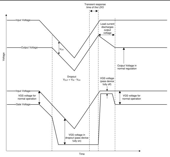
图 8-2. Line Transients From Dropout
