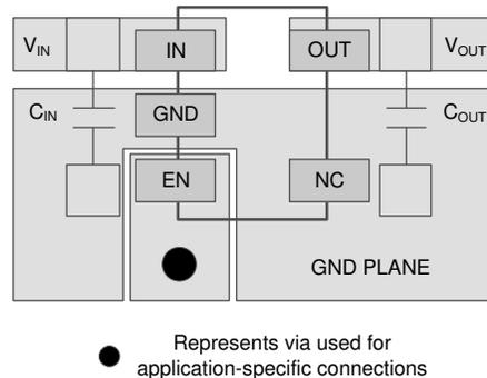
图 10-2. Layout Example for the DBV Package
