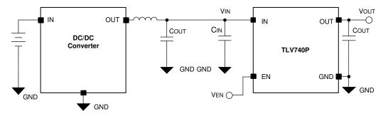
图 8-5. Operation From a DC/DC Converter
