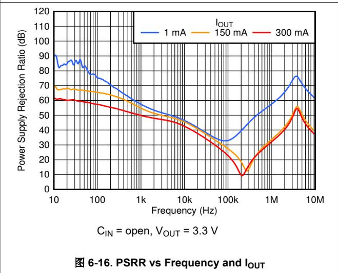
图 6-16. PSRR vs Frequency and  $I_{OUT}$
