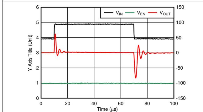
$V_{IN} = 3.9\text{ V}$  to  $4.9\text{ V}$ , slew rate =  $1\text{ V}/\mu\text{s}$ ,  $V_{EN} = 1\text{ V}$ ,  $I_{OUT} = 150\text{ mA}$
