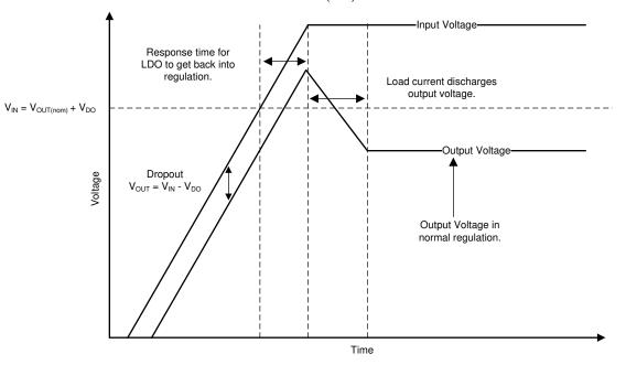
图 8-1. Start-Up Into Dropout
