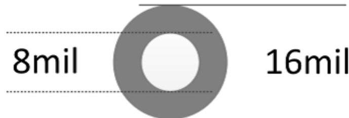
图 11-6. Recommended Minimum Via Sizing
