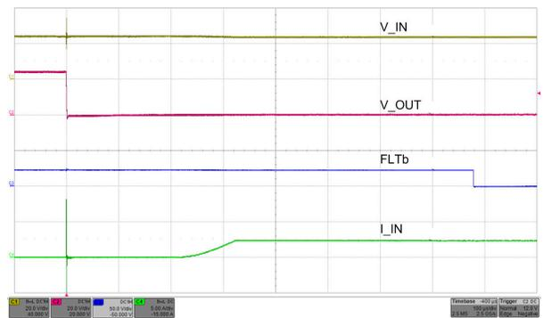
图 7-27. Hot-Short: Fast Trip Response and Current Regulation
