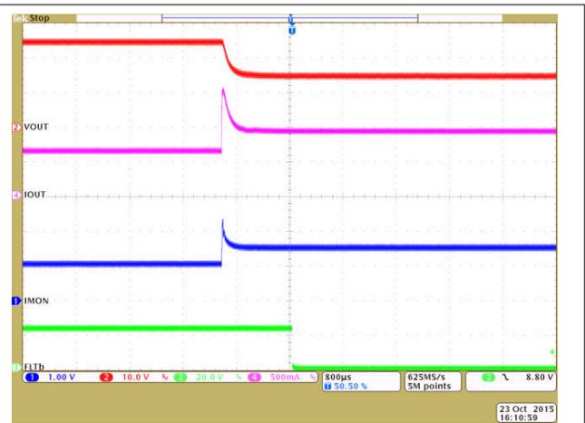
RILIM = 12 k $\Omega$       RILIM = 12 k $\Omega$       Load transient event
