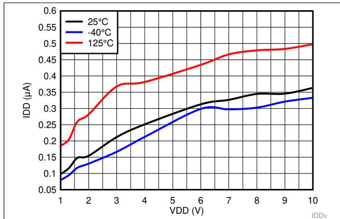
图 6. Supply Current vs Supply Voltage for TPS3840DL49
