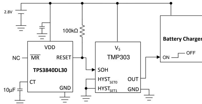
图 50. Overvoltage and Window Temperature Monitoring Solution
