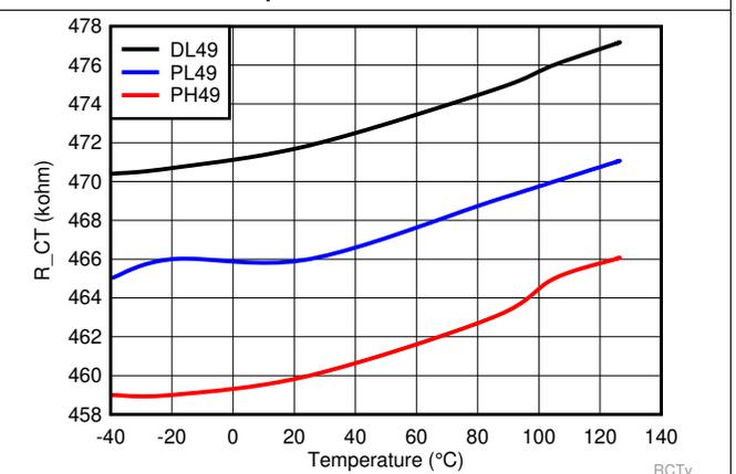
图 35. CT Pin Internal Resistance over Temperature
