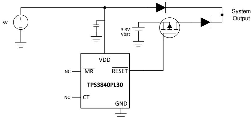
图 52. Voltage Monitor with Back-up Battery Switchover Solution
