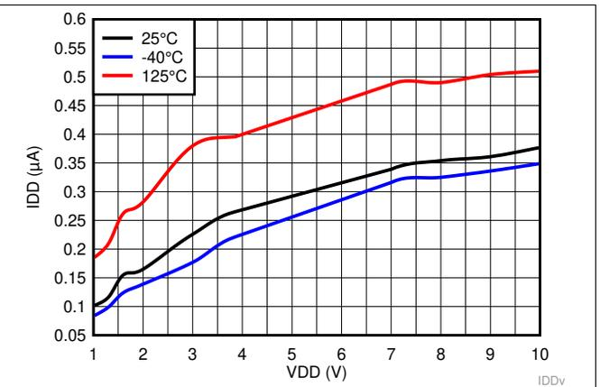
图 7. Supply Current vs Supply Voltage for TPS3840PL49
