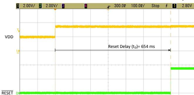
图 55. TPS3840EVM  $\overline{\text{RESET}}$  Time Delay ( $t_D$ ) with 1- $\mu\text{F}$  Capacitor
