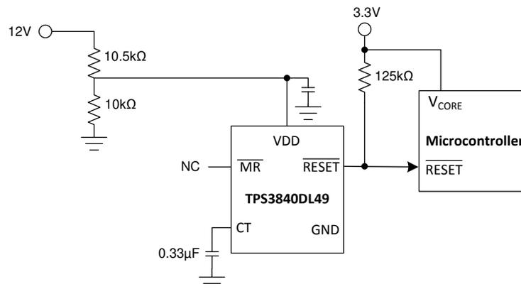
图 51. Fast Start Undervoltage Supervisor with Level-shifted Input
