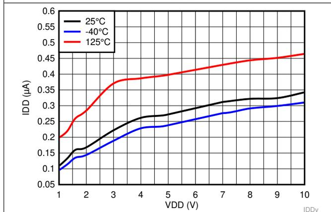
图 8. Supply Current vs Supply Voltage for TPS3840PH49
