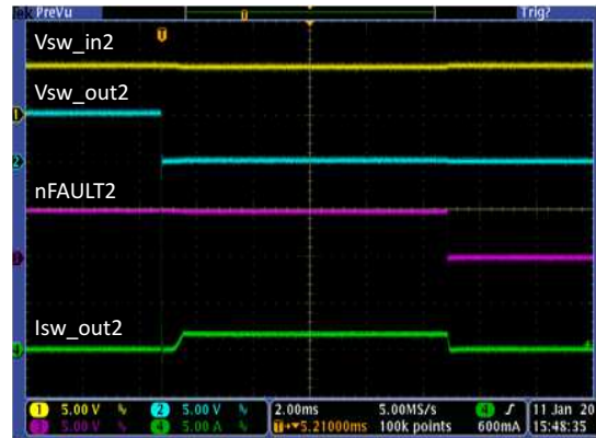
Figure 31. Power Switch2 Current Limit Operation
