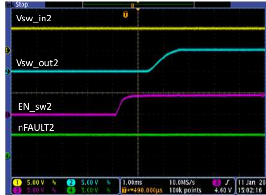
Figure 25. Power Switch2 Turn On Delay and Rise Time
