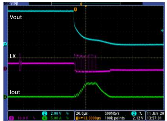
Figure 21. Zoom in Buck Output Hard-Short Response
