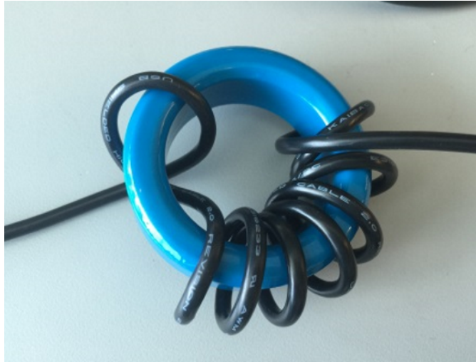
图 17. USB Cable Around Ferrite Bead
