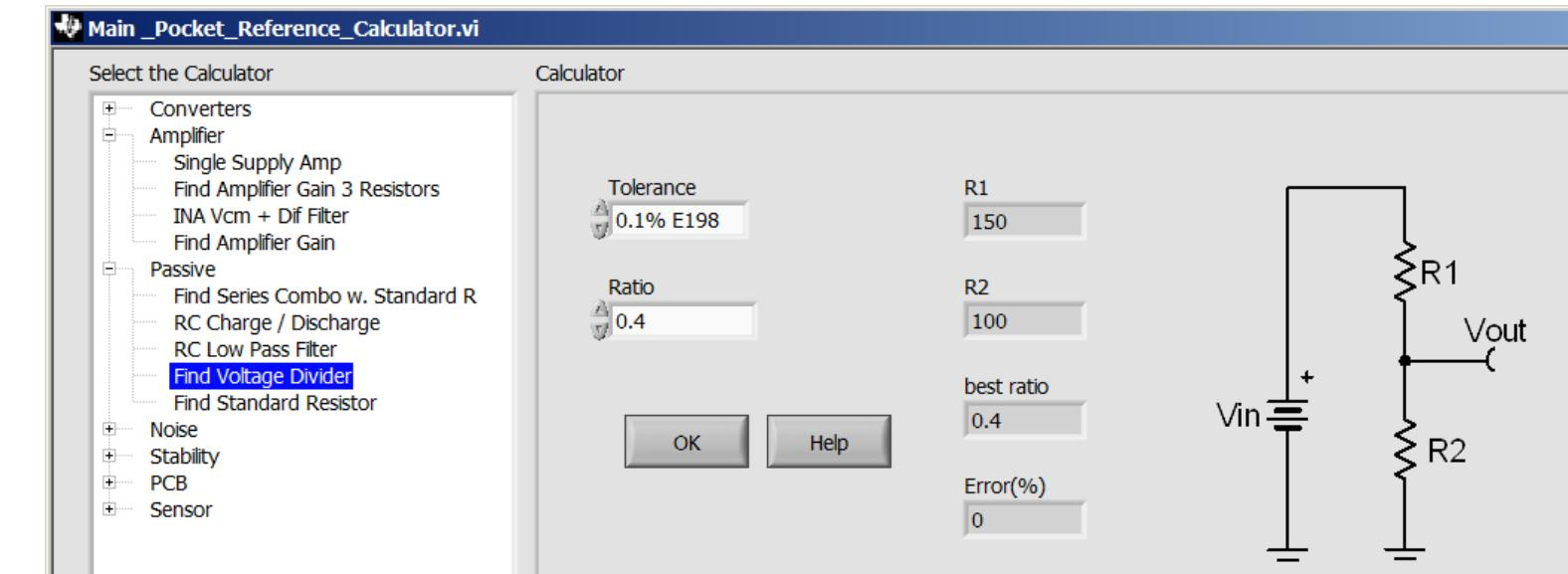
Use the calculator as simple way to find the voltage divider resistors.
