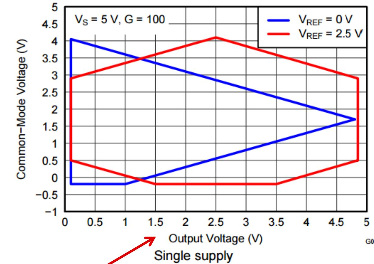
Figure 12. Input Common-Mode Voltage vs Output Voltage
