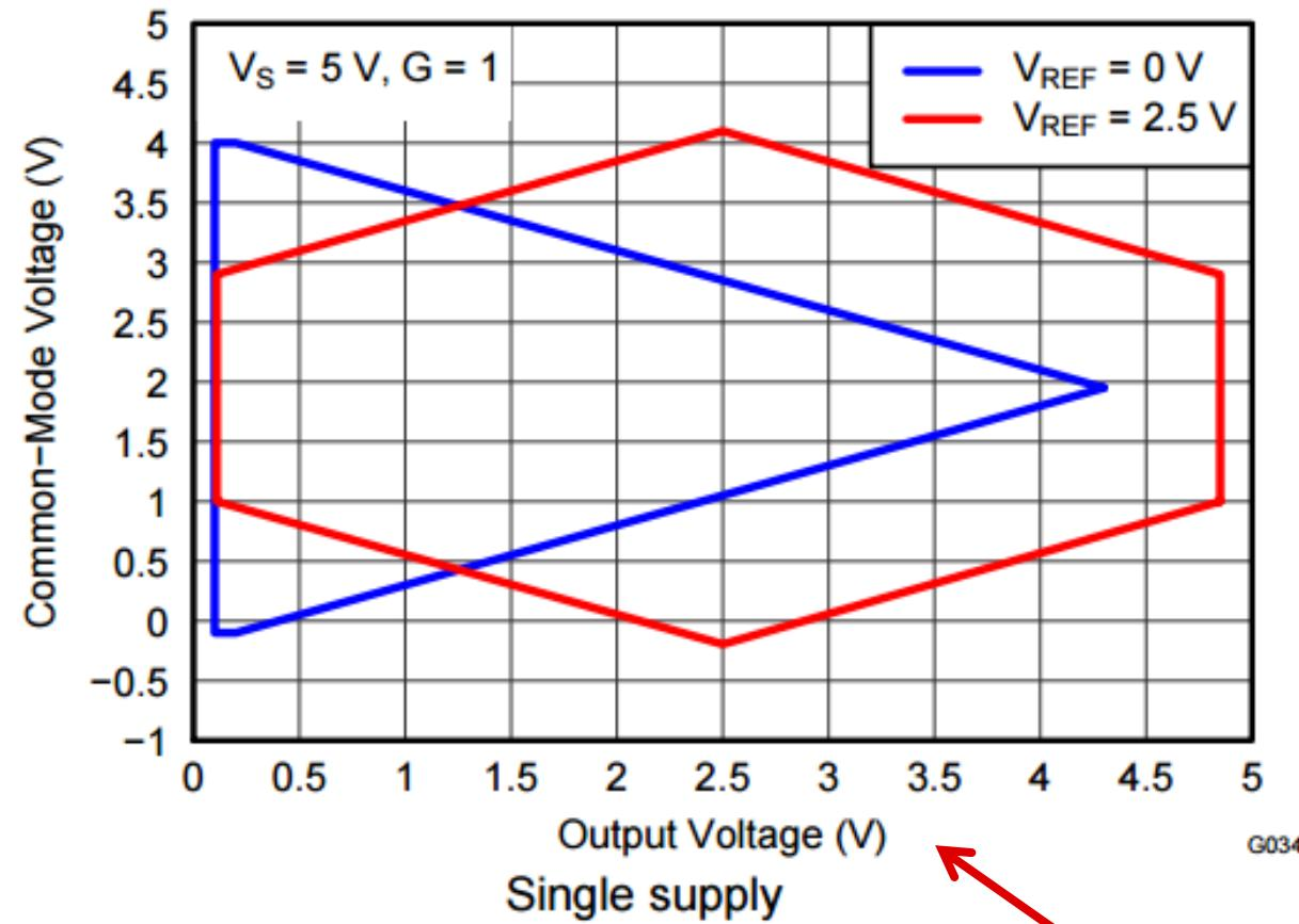
Figure 11. Input Common-Mode Voltage vs Output Voltage
