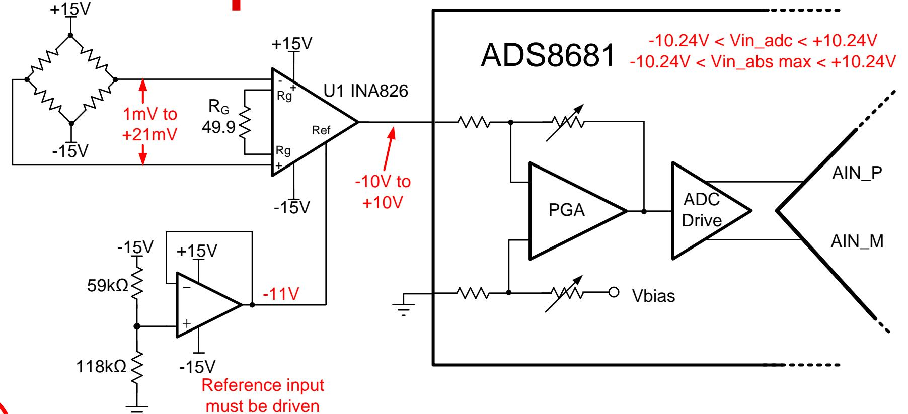
$$G_{826} = \left( \frac{\Delta V_{OUT}}{\Delta V_{IN}} \right) = \left( \frac{10V - (-10V)}{1mV - (-21mV)} \right) = 1000$$
