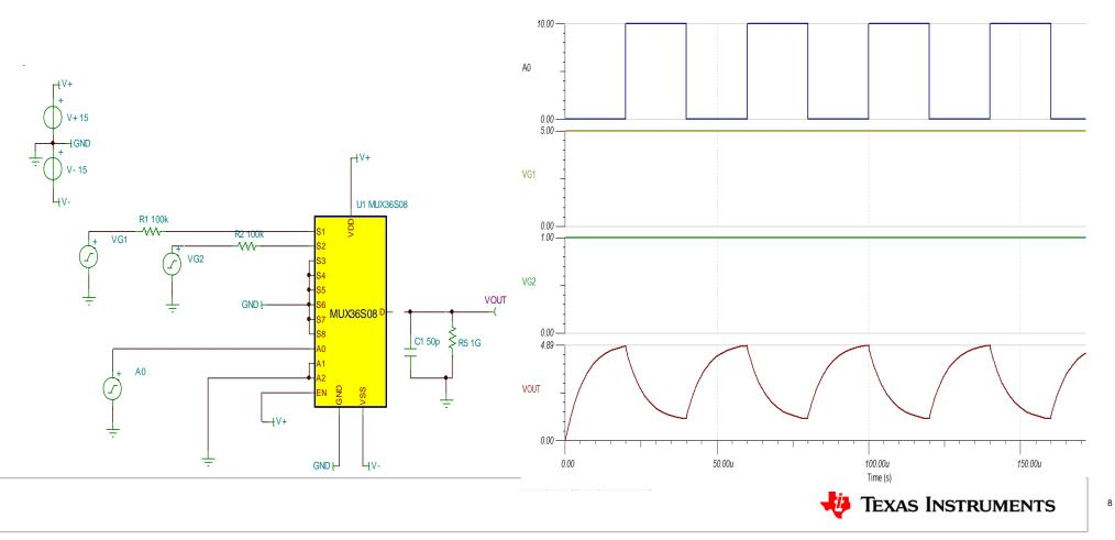
2. In the below circuit, the multiplexer input channels are fed with two high-impedance voltage sources. VG1 and VG2 have a DC output of 5V and 1V. The MUX has total on capacitance of 50pF. These channels are switched at 20us. Does the output settle to the input voltage in the given time period? Simulate it using TI-TINA.
