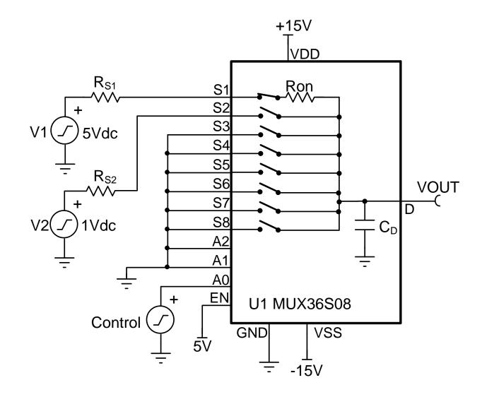
Charge on Capacitance C<sub>D</sub> when Channel-1 is ON :
