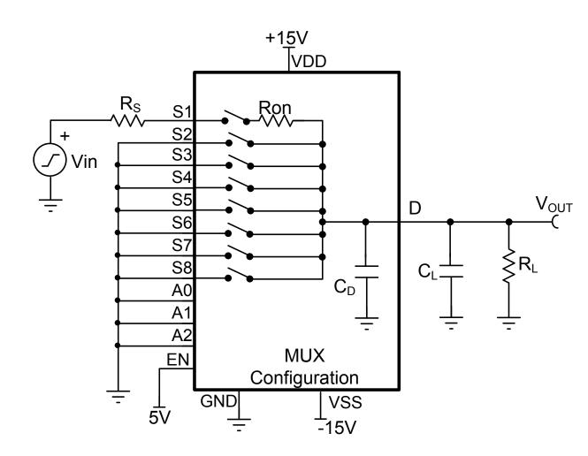
**OFF Isolation:** voltage at output pin of an multiplexer when a known signal is applied at the source pin of an OFF-channel
