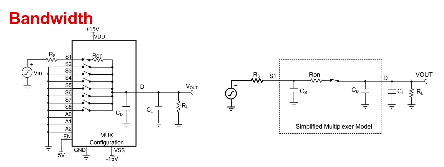
**Bandwidth** : The frequency at which the output is attenuated by 3 dB from the pass band (dc) response.
