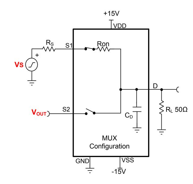
**Crosstalk:** voltage feed through to the source pin of an off-channel from a known signal is applied to the source pin of an on-channel
