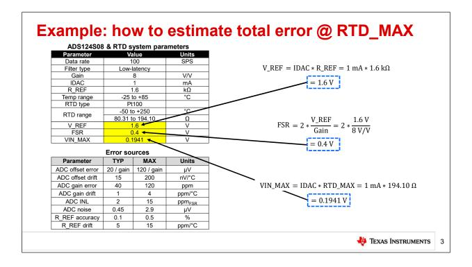
For this example, we will select the ADS124S08 to measure the RTD. This ADC is a 24-bit, 13 channel delta-sigma ADC with an integrated amplifier and current sources that is commonly-used for RTD measurements.
