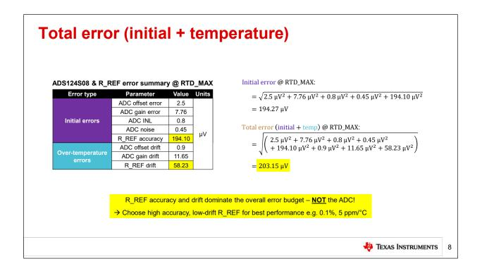
Before calculating total error, let's recall the initial error values and the total initial error derived previously in this presentation. The initial error values are highlighted in purple in the table on the left, while the total initial error is shown in the equation on the top right.
