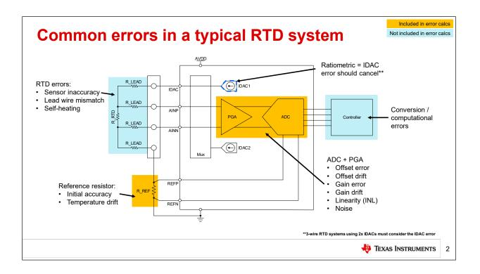
Shown here is a typical RTD measurement system that includes a 4-wire RTD connected to a terminal block, a low-side reference resistor, an ADC with an integrated PGA and current sources, and a controller to perform the resistance to temperature conversion. As discussed in a previous Precision Labs module, this system has several common error sources
