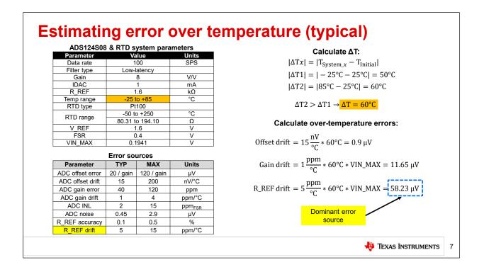
On the previous slide we calculated the maximum temperature change, delta T, for the system parameters included in the table on the top left. These calculations are shown on the top right, where delta T is 60 degrees Celsius. Now let's calculate the over temperature errors
