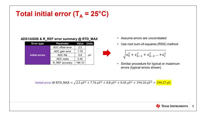
The table on the left summarizes the errors calculated in the previous slides. Use the following information to calculate total initial error
