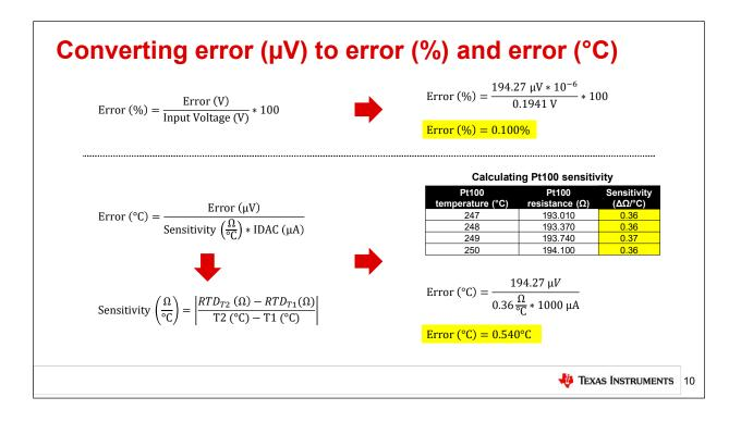
Throughout this presentation we've talked about error using different units, including microvolts and percent. Now let's discuss how to convert between these units. We'll also identify how to calculate error in degrees Celsius, which is a common requirement in RTD measurement systems
