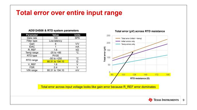
On the left are the ADC and system settings we have been using throughout this example. In the last slide we calculated the initial error, temperature error, and total error at the maximum RTD resistance of 194.1 ohms. Let's perform that same analysis across the entire input range
