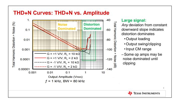
Let's take a close look at the distortion region. In this region, the distortion harmonics are greater than the rms noise voltage. Distortion harmonics can result from output loading, limitations in the output swing, or input common mode range violations. By inspection, we can tell that the slight increase in distortion is likely due to output loading, and we notice that the 2kOhm curves increase before the 10kOhm curves.
