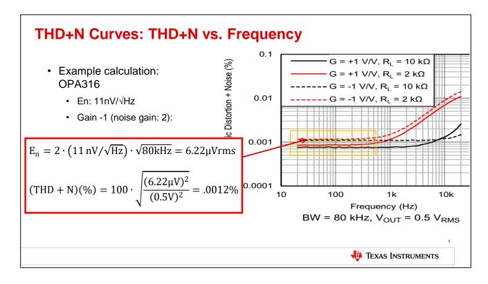
If you know the broadband noise spectral density of an op-amp you can do a simple calculation for the THD+N value in the noise dominated region. For the OPA316 example, the broadband noise spectral density is 11nV/rtHz from the data sheet. If we examine the gain equal to minus one case, then the noise gain of is 2V/V.
