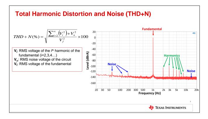
Total harmonic distortion and noise (THD+N) is a figure of merit that seeks to quantify the amount of unwanted content added to a signal by a circuit's noise and non-linearity. This can be important in audio systems, vibration analysis systems, data acquisition systems, and many other applications.
