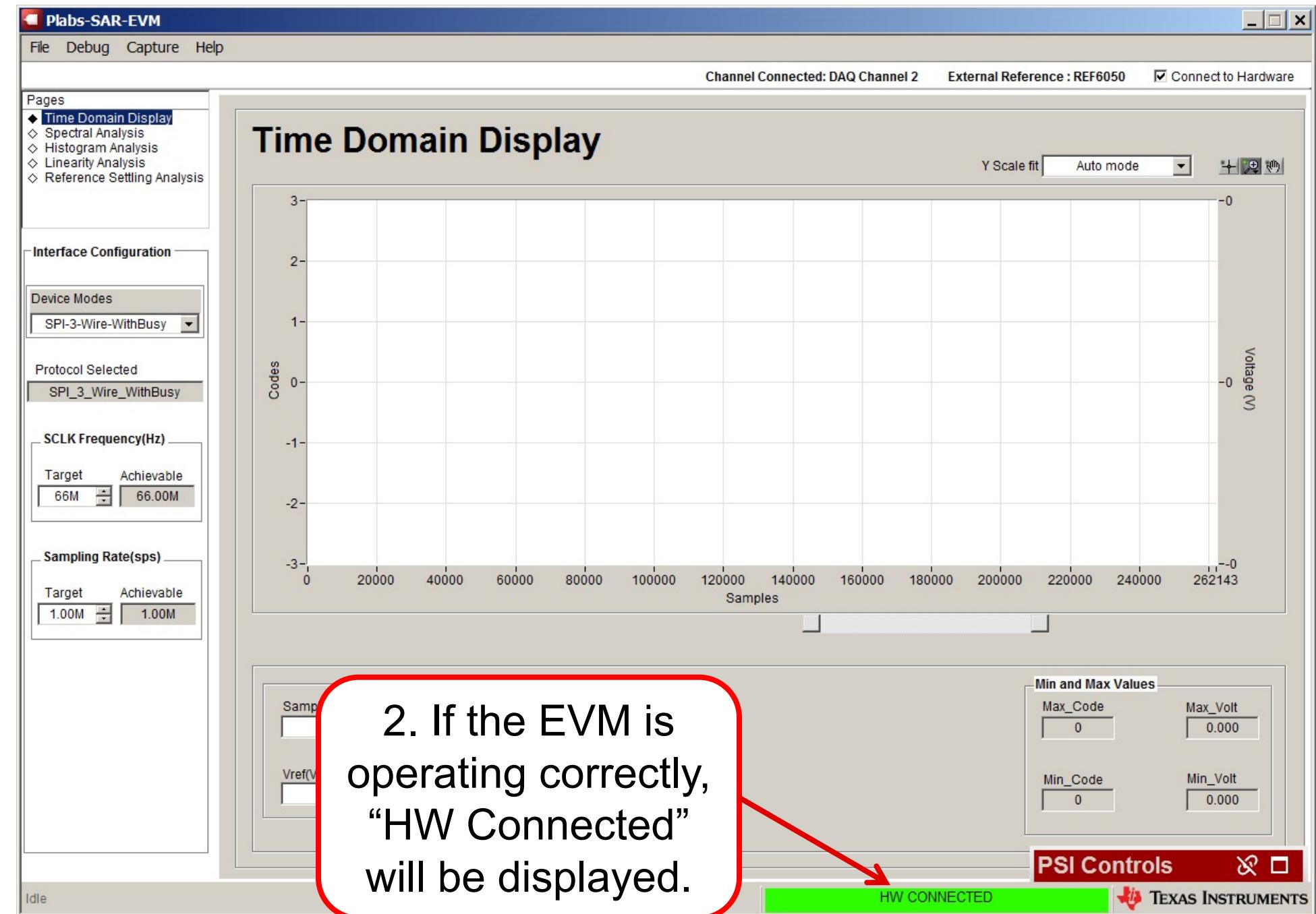
2. If the EVM is operating correctly, “HW Connected” will be displayed.
