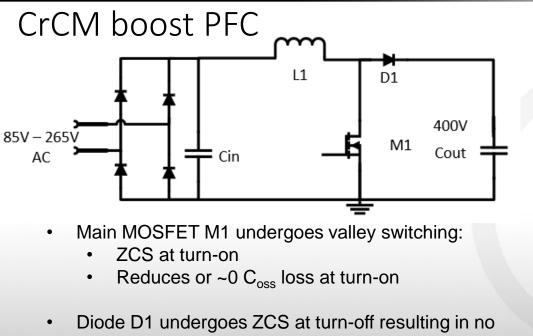
Diode D1 undergoes ZCS at turn-off resulting in no
