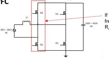
If we replace the low frequency diode with low R<sub>dson</sub> MOSFET
