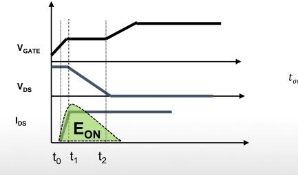
$t_{on} = t_{1} + t_{2}$   $t_{on} = \left(\frac{Q_{gd}}{V_{ds}}\right) * Rgate * \left(\frac{V_{ds} - Vpl}{V_{gate} - Vpl}\right) + Ciss * Rgate * Ln(\frac{V_{gate} - Vth}{V_{gate} - Vpl})$   $Pon_{overlap} = 0.5 * Vds * IHV_{on} * ton * Fsw$
