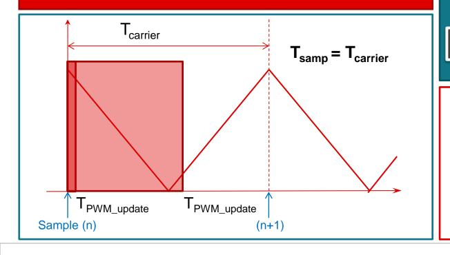
Try to make  $T_{PWM\_update} < 1\% \text{ of } T_{samp}$
