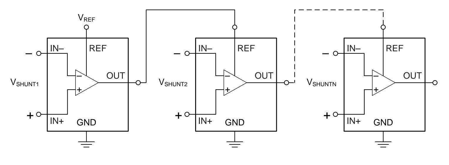
$V_0 = (V_{shunt1} + V_{shunt2} + \dots + V_{shuntn}) * Gain + V_{ref}$
