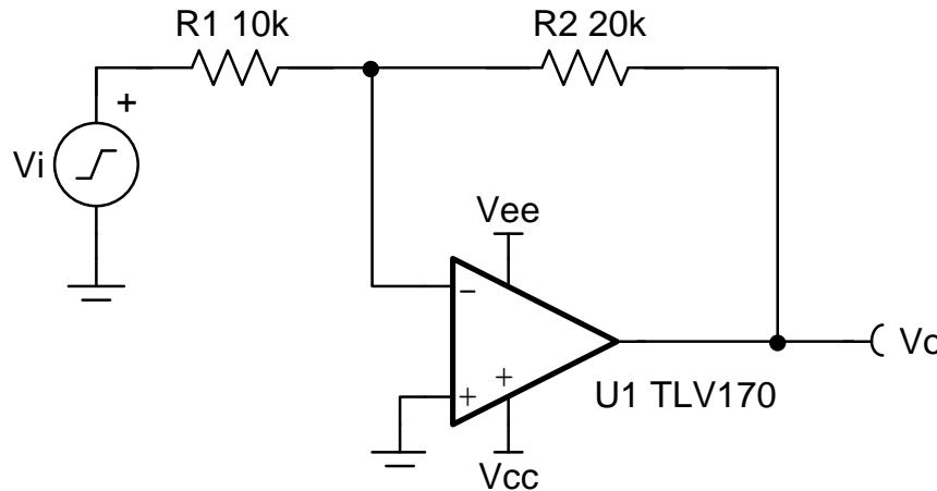
$$G = \frac{V_{oMax}}{V_{iMin}}$$
