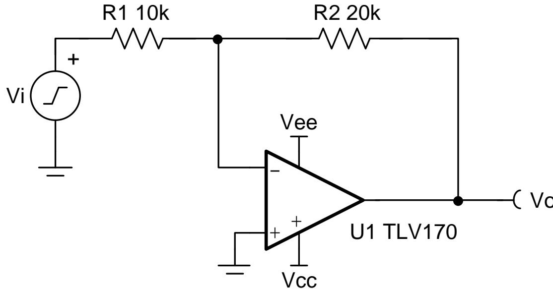
$$V_o = -\frac{R_2}{R_1} \times V_i$$
