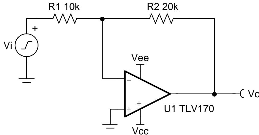
$$V_o = -\frac{R_2}{R_1} \times V_i$$
