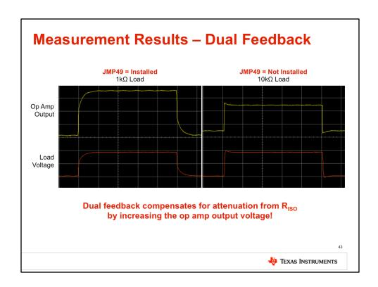
You should see results similar to this. As you can see, the load voltage remains accurate, even with changing load, due to the compensation provided by the dual-feedback network. The unloaded op-amp output voltage must increase as the load resistance decreases to minimize the output voltage divider effect.
