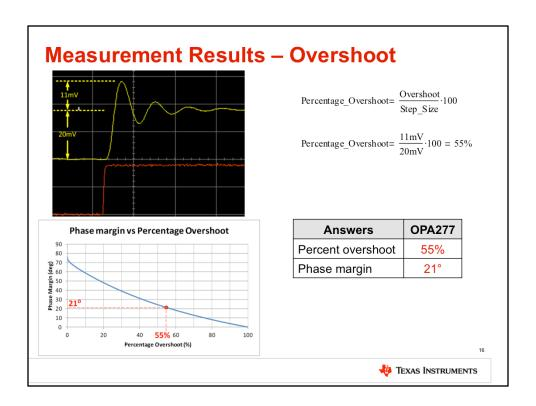
Use cursors to measure the amount of overshoot. The expected measurement results are shown here. The measured overshoot of 55% results in a phase margin of 21 degrees. Your results may vary slightly.
