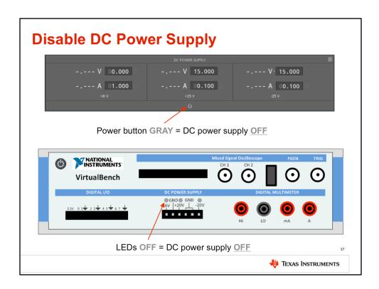
Make sure to disable the DC power supply before setting up the test PCB! In the VirtualBench software, click the power button in the DC Power Supply area to turn off the power. Check the front panel of the VirtualBench unit to make sure the LEDs are OFF! Also ensure the function generator is OFF.
