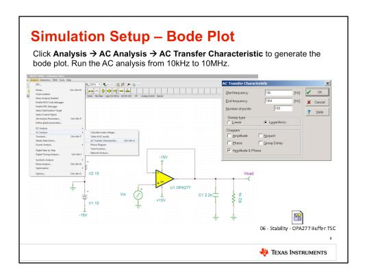
Next, run a SPICE simulation analysis for the AC transfer characteristic. This will allow us to see the op amp's AC peaking, which is another indicator of phase margin.
