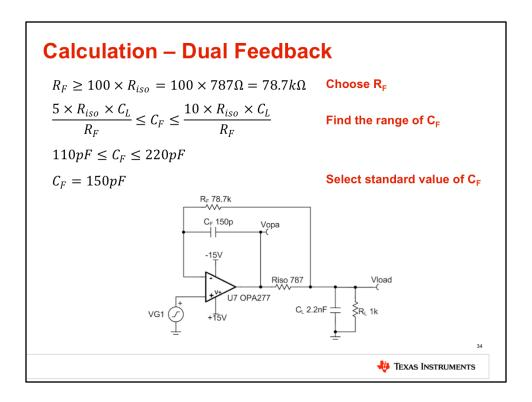
To select the components of the dual feedback network, use the equations given on this slide. For this example, Rf was chosen to be 78.7k, and Cf was chosen to be 150pF.
