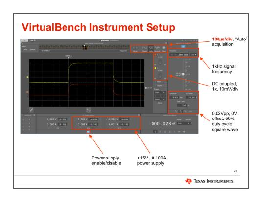
The VirtualBench setup is almost the same as before. Only change the time scale to 100us/div. All other settings must remain the same.
