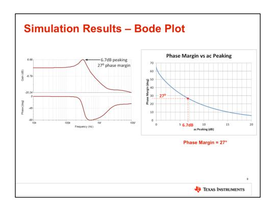
You should see a result similar to this. The 6.7dB of simulated AC peaking results in a phase margin of approximately 27 degrees.
