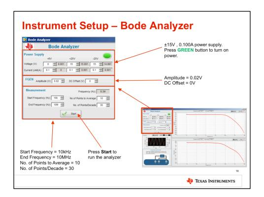
In the configuration panel, set the power supply to  $\pm 15$ V, 0.1A. Press the green button to turn on the power.
