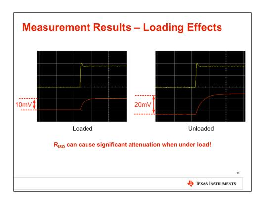
As you can see, the load voltage changes dramatically if the circuit is loaded or unloaded! In fact, when loaded, the circuit with Riso shows attenuation of approximately 50%! This is simply due to the voltage divider effect of Riso and the load resistance.
