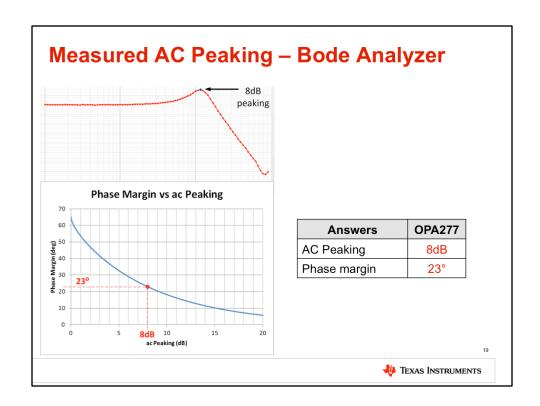
You should see a result similar to this. Enable the cursor, then drag the cursor to the maximum value to measure the AC peaking. In this measurement, AC peaking of 8dB resulted in a phase margin of 23 degrees. Your results may vary slightly.
