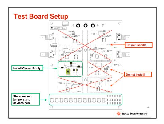
The test board setup remains the same as before. Install circuit 5 only, and store any unused jumpers and devices in the storage area at the bottom of the test board.
