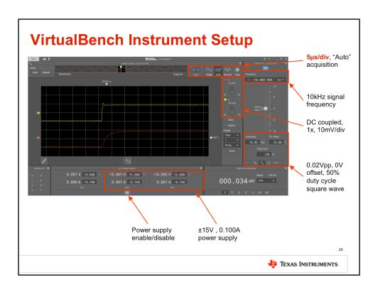
The VirtualBench setup is almost the same as before. Only change the time scale to 5us/div. All other settings must remain the same.
