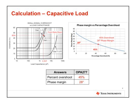
This circuit uses the OPA277. In order to perform the calculations, you need to know the percent overshoot versus load capacitance for that device, shown on the top left. Then, use the plot on the right to determine the phase margin from that percentage overshoot.
