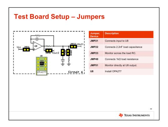
To prepare the test board for the measurement, install the jumpers and devices on circuit 6 as shown here.
