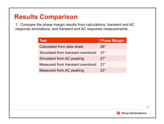
Now, compare the phase margin results from your hand calculations, transient and AC response simulations, and transient and AC response measurements. While there is some slight variation to the results, the phase margin values compare very well at approximately 27 degrees.
