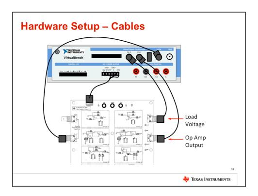
This slide gives the new connection diagram between the TI Precision Labs test board and the National Instruments VirtualBench. Connect the provided power cable to the DC power supply of the Virtual Bench and power connector J4 on the test board.
