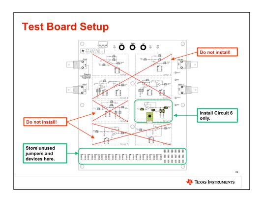
For the test board to function properly, it is important that you only install jumpers and devices in circuit 6! Do not install any jumpers or devices in any other circuits on the PCB! Remove any jumpers or devices from the unused circuits and store them in the storage area at the bottom of the test board.
