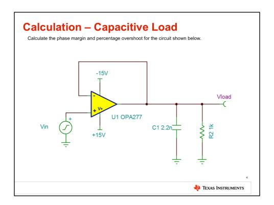
First, calculate the phase margin and percentage overshoot for the circuit shown here, using the techniques and equations given in the stability lecture. Use the plots given on the next slide.
