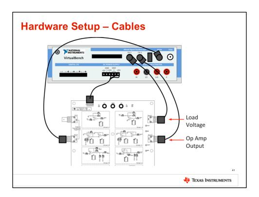
The cable connections are the same as in Experiment 2. Connect the provided power cable to the DC power supply of the Virtual Bench and power connector J4 on the test board.
