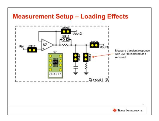
As an additional experiment, measure the transient response again with JMP48 installed and removed. This will connect and disconnect the 1k load resistor from the circuit.
