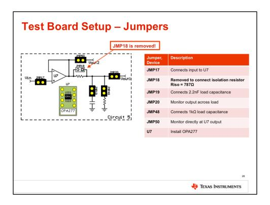
Let's now re-run the overshoot measurement, this time with Riso. The jumper setup is almost the same. The only change is to remove JMP18, which connects the isolation resistor of 787 ohms.
