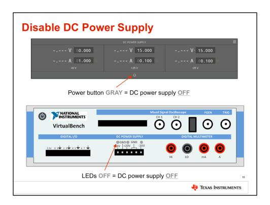
Make sure to disable the DC power supply before setting up the test PCB! In the VirtualBench software, click the power button in the DC Power Supply area to turn off the power. Check the front panel of the VirtualBench unit to make sure the LEDs are OFF! Also ensure that the function generator is OFF.
