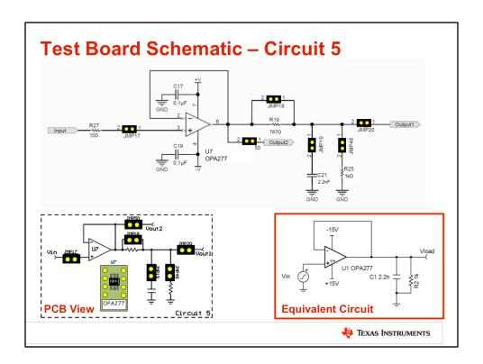
This slide shows the full schematic for Circuit 5 on the TI Precision Labs test board. You will use this circuit to measure the stability of the OPA277.
