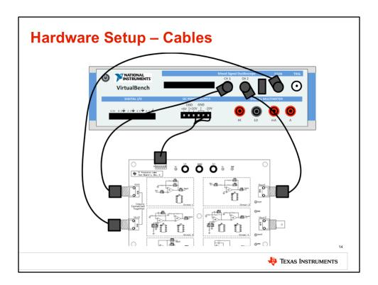
This slide gives the connection diagram between the TI Precision Labs test board and the National Instruments VirtualBench. Connect the provided power cable to the DC power supply of the Virtual Bench and power connector J4 on the test board.
