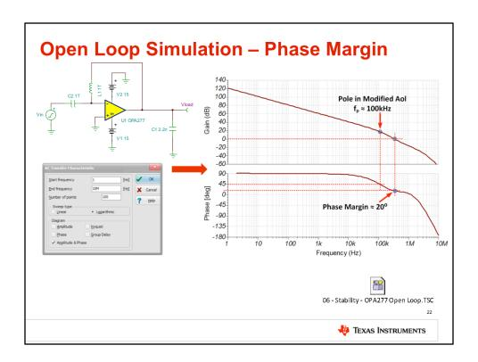
To determine the value of isolation resistor Riso, we must first know the open-loop AC response of the circuit. Here we show the TINA-TI simulation schematic and AC response results, which you can verify using the embedded file.
