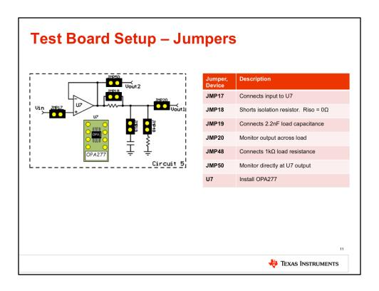
To prepare the test board for the measurement, install the jumpers and devices on circuit 5 as shown here.
