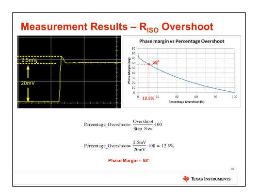
Use cursors to measure the amount of overshoot. You should see results similar to this. With Riso, the measured unloaded output overshoot was reduced to 12.5%, resulting in a phase margin of approximately 58 degrees which indicates a stable circuit.
