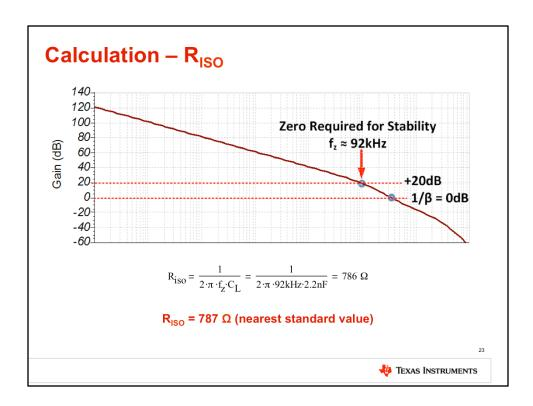
For best results, Riso should create a zero in the loop response 20dB greater than the frequency where the open-loop gain intersects with the closed-loop gain. This circuit is a buffer with a closed-loop gain of 0dB, so the zero should occur at 20dB. The open-loop gain is equal to 20dB at 92kHz. Use this value and the load capacitance to calculate Riso, which is 786 ohms in this example. 787 ohms is the nearest standard value resistance.
