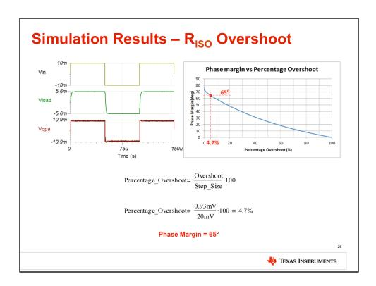
You should see results similar to this. With Riso added to the circuit, the overshoot was reduced to only 4.7%. This results in a phase margin of 65 degrees, indicating a stable circuit.
