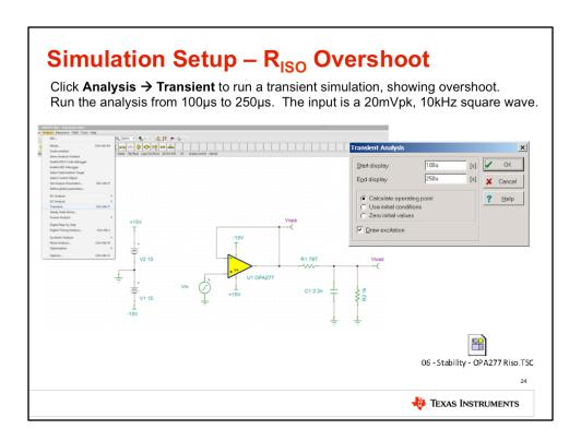
Let's now simulate the transient overshoot with Riso included in the circuit. As before, click Analysis → Transient to run the simulation. Run the analysis from 100us to 250us. The input is a 20mVpk, 10kHz square wave.
