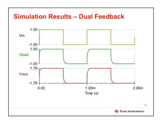
You should see results similar to this. As you can observe, in this configuration the loaded output voltage matches very well with the input. To achieve this, the unloaded output voltage Vopa must increase to compensate for the attenuation caused by Riso and the load resistance.
