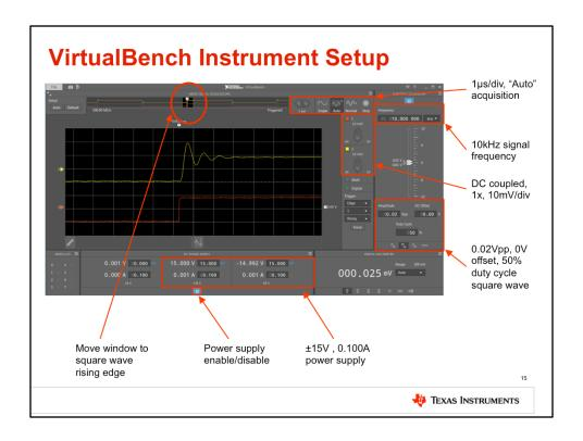
Next apply power to the National Instruments VirtualBench and connect it to your computer with a USB cable. The hardware should be detected as a virtual CD drive, and you can run the VirtualBench software directly from the drive. Once the software opens, configure the software as follows:
