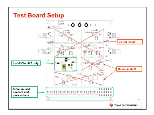
For the test board to function properly, it is important that you only install jumpers and devices in circuit 5. Do not install any jumpers or devices in any other circuits on the PCB! Remove any jumpers or devices from the unused circuits and store them in the storage area at the bottom of the test board.
