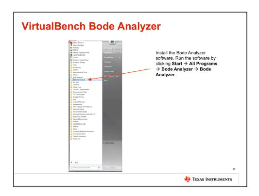
This lab requires additional Bode analyzer software. Install the software, then run it by clicking Start  $\rightarrow$  All Programs  $\rightarrow$  Bode Analyzer  $\rightarrow$  Bode Analyzer.
