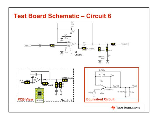
This slide shows the full schematic for Circuit 6 on the TI Precision Labs test board. You will use this circuit to measure the transient behavior of the OPA277 in a dual-feedback configuration.
