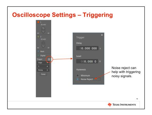
The icon at the top right of the trigger settings opens a new window with more trigger options. The trigger time delay and voltage level can be set. Leave these both at zero. Hysteresis is also available to help with triggering noisy signals. Try both options, but for this lab use "noise reject" mode.
