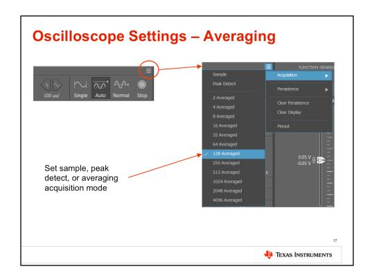
The icon at the top right of the acquisition settings opens more acquisition options. The acquisition mode can be changed to sample, peak detect, or average. Set the acquisition to 128 times averaged.
