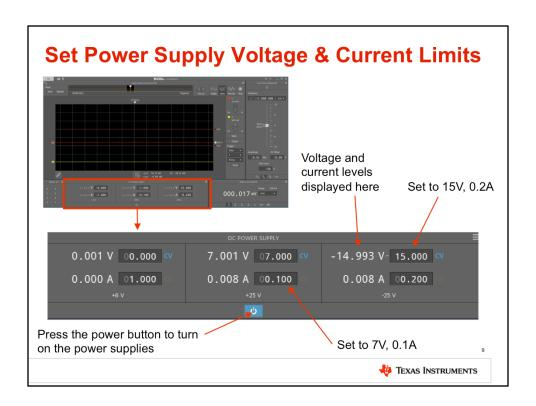
Once the software opens, let's first set the power supply voltage and current limits. Set the +25V supply to +7V, 0.1A. Set the -25V supply to -15V, 0.2A. Press the blue power button to turn on the power supplies.
