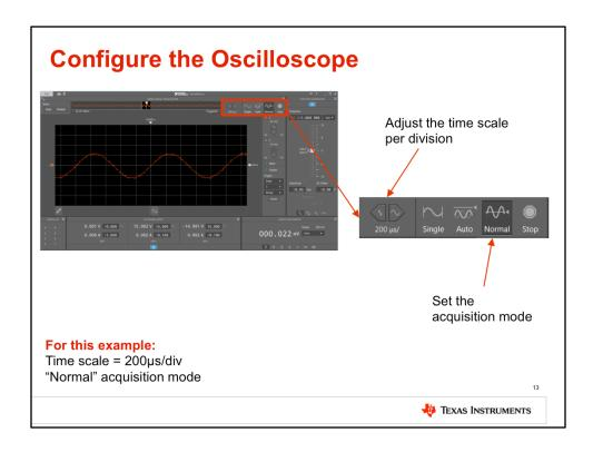
Let's now configure the oscilloscope. The overall acquisition and display settings are configurable. Adjust the time scale to  $200\mu s/division$ . Set the acquisition mode to "Normal."
