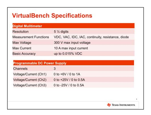
The specs are continued here for the multimeter and power supply. The multimeter has 5 and a half digits of resolution, and the three-channel power supply can support both single supply and split supply devices.
