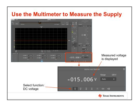
In the software, select the DC voltage function of the multimeter at the bottom right. The measured voltage will now be displayed in the large white text. It should read -15V, the same as what was configured.
