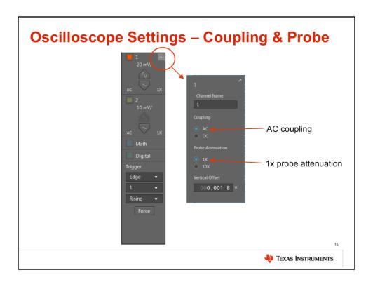
The icon at the top right of the oscilloscope opens a new window with more options for each channel. Each channel can be given a custom name. Set the coupling mode to AC. Set probe attenuation to 1x.
