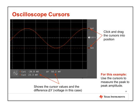
The cursors location may be adjusted to make a measurement. Click and drag the cursor indicators into position at the top and bottom of the sinusoidal waveform. The voltage level at each cursor, as well as the delta Y, in this case voltage difference, will be displayed next to the cursor icon. Use the cursors to measure the signal's peak-to-peak amplitude. You should see a result of 50mVpp, the same amplitude as the function generator.
