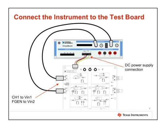
Let's now make some connections between the VirtualBench and the Test Board. Use the included cable to connect to the DC power supply. Use a BNC cable to connect CH1 of the VirtualBench oscilloscope to Vin1 on the test board. Use another BNC cable to connect the VirtualBench function generator, labeled FGEN, to Vin2 on the test board.
