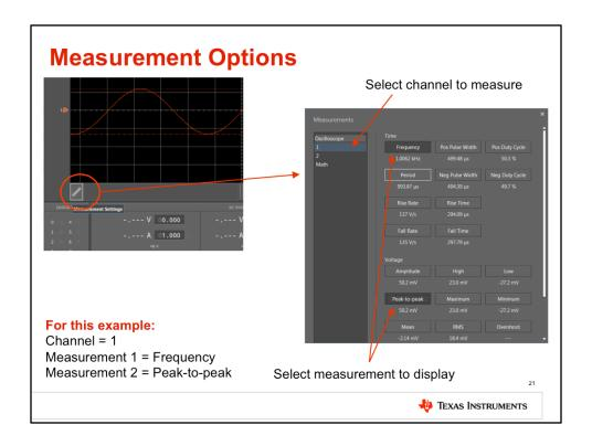
The VirtualBench can also make measurements automatically. Click the ruler icon, above the digital I/O settings, to open the measurement options window. Here you can select what channel to measure, and which measurement you want to display. Select channel 1, and measure both frequency and peak-to-peak amplitude.
