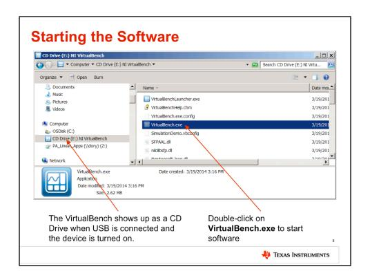
The VirtualBench software is pre-installed on the device. Once power is applied and USB is connected, you can see the VirtualBench as a CD drive. Click the drive, then double-click VirtualBench.exe to start the software.
