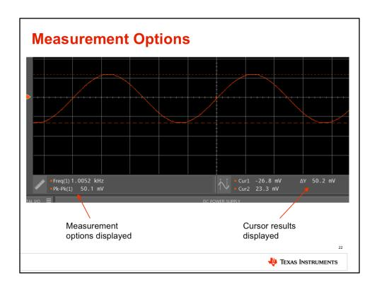
The measurement results are displayed next to the ruler icon. You should read a result of 1kHz, 50mVpp – the same as the function generator. The amplitude should be the same as the delta Y measurement from the cursor.
