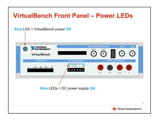
The front panel of the VirtualBench also has several power LEDs. The power button on the top left of the unit will glow BLUE when the VirtualBench is on. 3 LEDs in the DC Power Supply area will also glow blue when the DC Power Supply is on.
