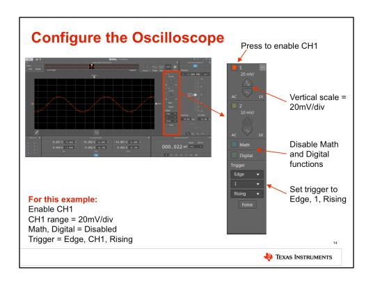
Press the red button to enable CH1. Set the voltage range to 20mV/div. Leave math and digital functions disabled. Set the trigger to Edge, CH1, Rising.
