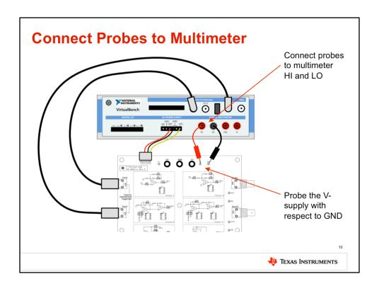
Let's now measure the power supplies that we just configured. To do this, we'll use the built-in multimeter. Connect the included probes to the HI and LO inputs on the multimeter. Probe the V- supply with respect to GND, by touching the red probe to V- and the black probe to GND.
