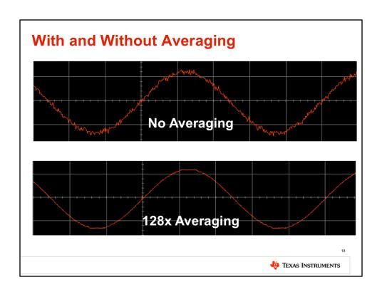
When measuring periodic signals, averaging can help significantly reduce the amount of noise displayed on the measured signal. This slide shows the difference between no averaging, or "sample" mode, and 128 times averaging.
