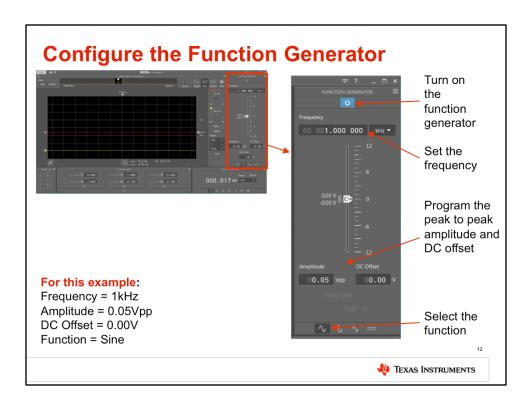
Next, we'll configure the function generator. First, set the frequency to 1kHz. Then, adjust the amplitude to 0.05Vpp with 0V DC offset. Select the sinusoidal function. Finally, press the blue power button to turn on the function generator.
