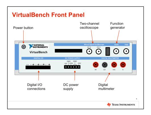
The front panel of the virtual bench is used to make connections to your system under test. You must turn on the VirtualBench by pressing the power button on the top left before using the device. Then, you can connect to the oscilloscope, function generator, digital I/O, DC power supply, and digital multimeter as required in your experiments.
