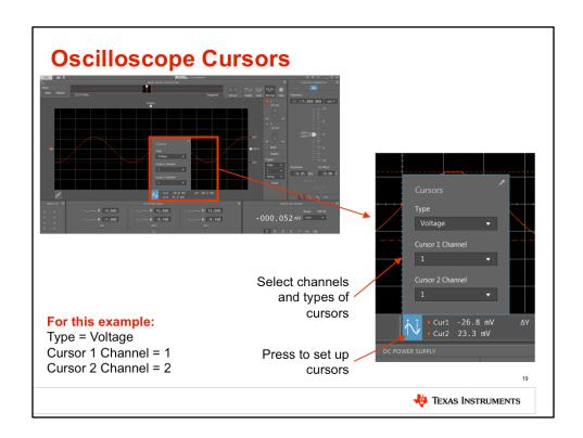
Cursors may be used to measured oscilloscope signals. Click the cursor icon, located above the power supply settings, to open the cursor menu. Select voltage type, then set Cursor 1 Channel to 1 and Cursor 2 Channel to 1.
