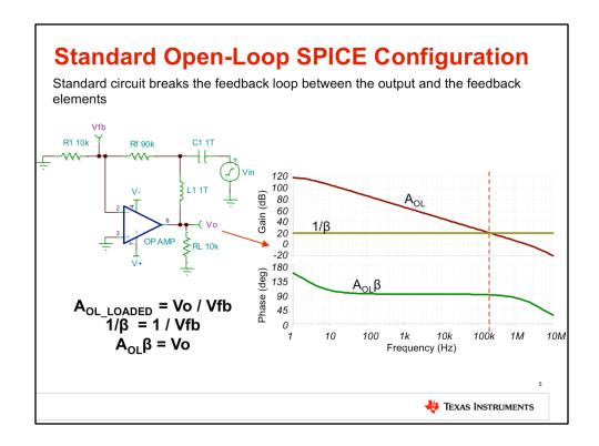
Therefore, here is the recommended standard open-loop SPICE circuit configuration for op amp circuits. The feedback loop is broken between the op amp output and the feedback elements. The ac signal source is injected into the feedback network and measurements are taken at the output, Vo, and feedback node, Vfb.
