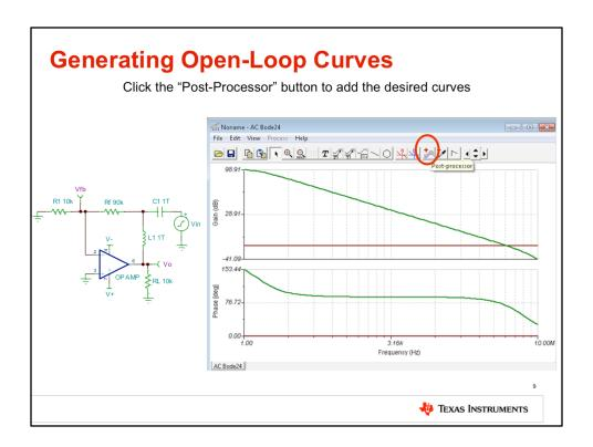
The results for the Vo and Vfb probes will be displayed after the simulation is complete. To add the desired curves for open-loop analysis, click the post-processor button in the result window.
