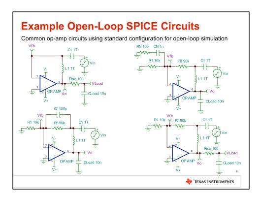
Several example circuits ready for open-loop simulation are shown here. They can be used for review if there is confusion regarding where to break the loop in many standard circuit configurations.
