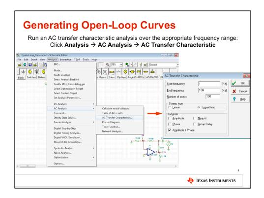
Once you've verified the dc operating point of the circuit, perform an ac transfer characteristic analysis over the op-amp bandwidth. Click Analysis, AC Analysis, AC Transfer Characteristic to do this.
