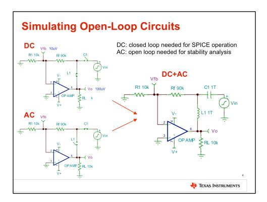
To properly generate the open-loop curves in SPICE, the circuit being simulated must have a closed loop feedback path at dc while being open for all ac frequencies.
