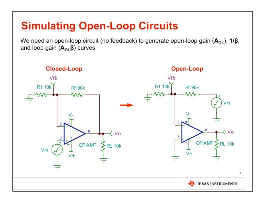
The AoI, 1/ß, and AoIß curves required for rate of closure and phase margin measurements can not be obtained from a circuit in a standard closed-loop configuration. To generate these curves, the feedback loop of the amplifier needs to be opened up, or "broken". Then, a small signal source is used to excite the high-impedance side of where the loop was broken. Measurements can then be taken at the op amp inverting input (Vfb) and output (Vo), which will be used to derive the desired curves.
