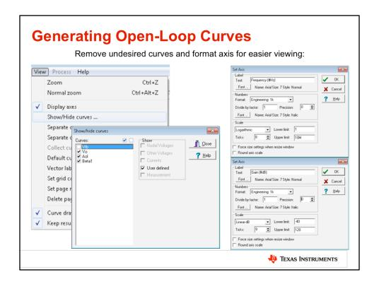
Click View, then Show/Hide curves. Select only the curves Vo, AoI, and Beta1. Then, double-click the x-axis and y-axis to bring up the "Set Axis" window. Change the x-axis to a logarithmic scale, 8 ticks, lower limit 1Hz, upper limit 10MHz. Change the y-axis to a linear-in-dB scale, 9 ticks, lower limit -40dB, upper limit 120dB.
