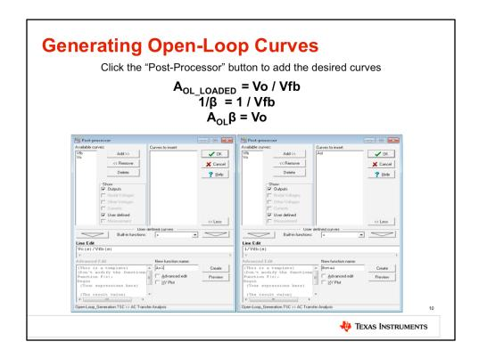
Write the proper equations for AoI and  $1/\beta$  in the line editor, name them, and then create the curves. A new curve can be added for AoI\* $\beta$ , but since it equals "Vo" which is already displayed, this is not necessary.
