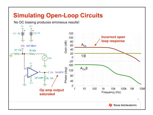
However, simply breaking the feedback loop of a circuit will not produce correct simulation results! Without a proper dc bias, the output will saturate to one rail or the other, reducing the performance of the output stage. As shown here, the op-amp output is near the positive rail, resulting in erroneous AoI and AoIß curves.
