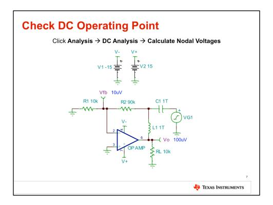
Before checking the ac behavior of the circuit, a quick check of the dc operating point should be performed. Simply click Analysis, DC Analysis, Calculate Nodal Voltages to do this. Vfb should show the input offset voltage, or Vos, of the op amp, while Vo will show Vos multiplied by the closed-loop gain.
