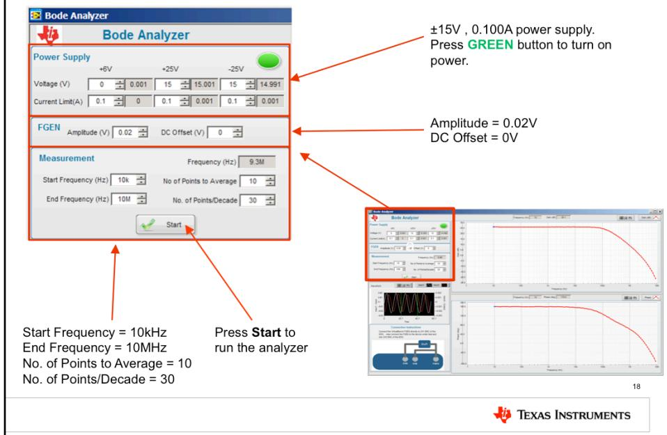
In the configuration panel, set the power supply to ±15V, 0.1A. Press the green button to turn on the power.
