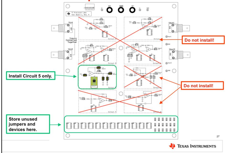
The test board setup remains the same as before. Install circuit 5 only, and store any unused jumpers and devices in the storage area at the bottom of the test board.
