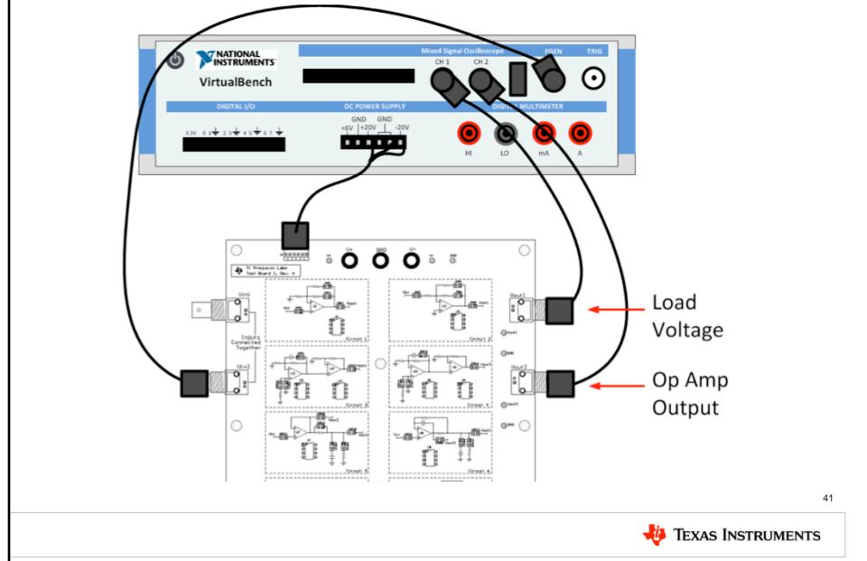
The cable connections are the same as in Experiment 2. Connect the provided power cable to the DC power supply of the VirtualBench and power connector J4 on the test board.
