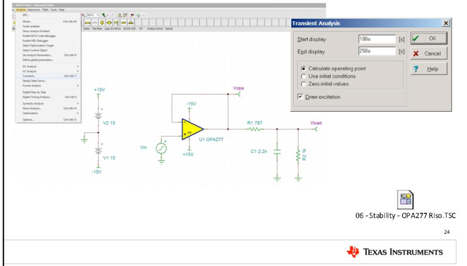
Let's now simulate the transient overshoot with Riso included in the circuit. As before, click Analysis → Transient to run the simulation. Run the analysis from 100 $\mu$ s to 250 $\mu$ s. The input is a 20mVpk, 10kHz square wave.
