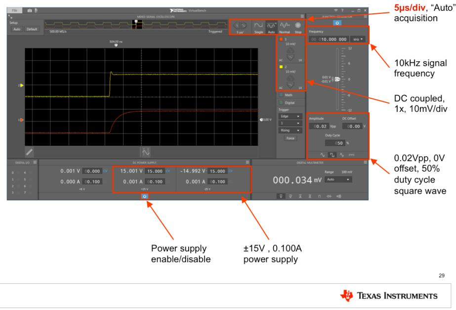
The VirtualBench setup is almost the same as before. Only change the time scale to 5 $\mu$ s/div. All other settings must remain the same.
