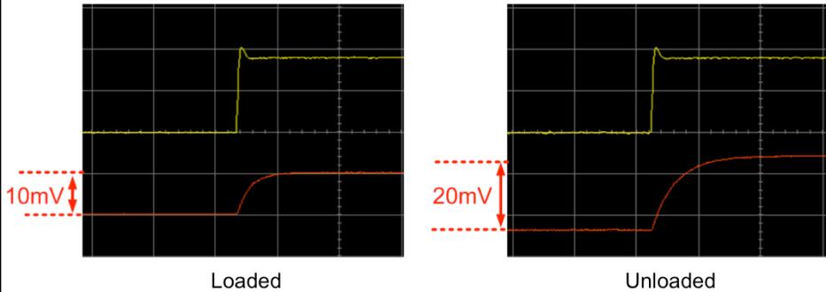
**R<sub>ISO</sub> can cause significant attenuation when under load!**
