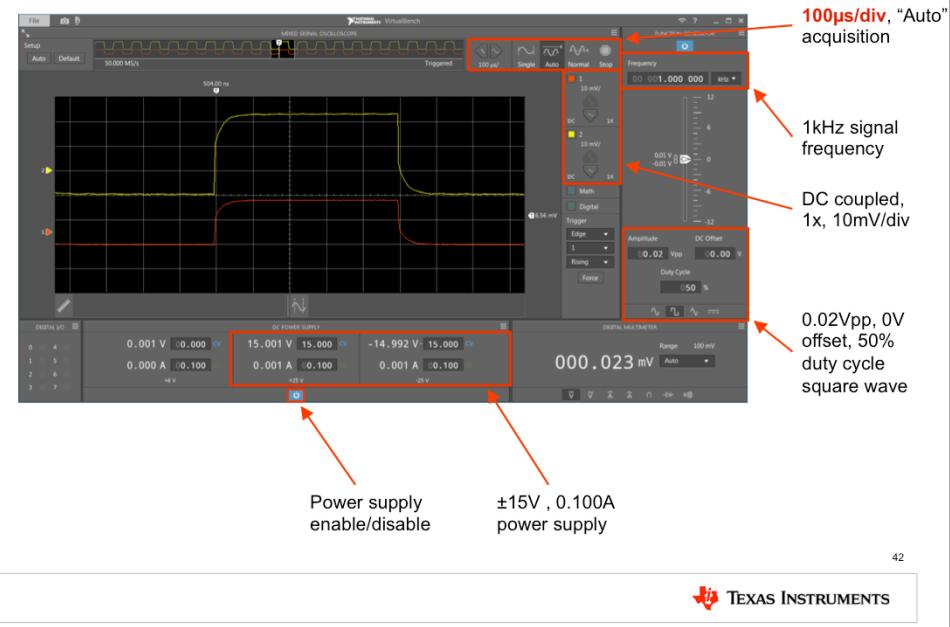
The VirtualBench setup is almost the same as before. Only change the time scale to 100μs/div. All other settings must remain the same.
