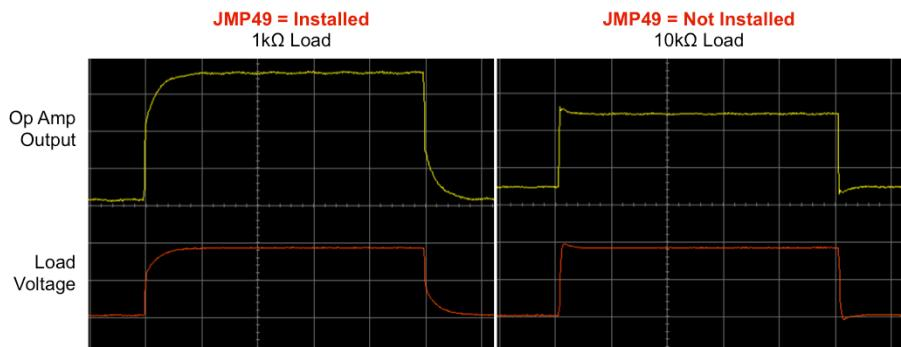
Dual feedback compensates for attenuation from  $R_{ISO}$  by increasing the op amp output voltage!
