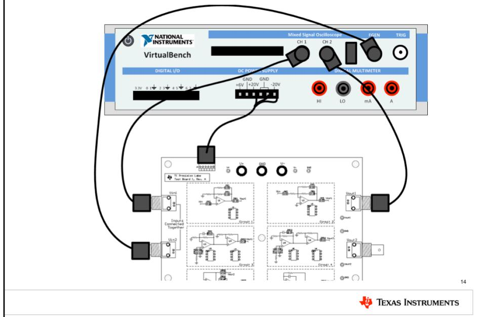
This slide gives the connection diagram between the TI Precision Labs test board and the National Instruments VirtualBench. Connect the provided power cable to the DC power supply of the Virtual Bench and power connector J4 on the test board.
