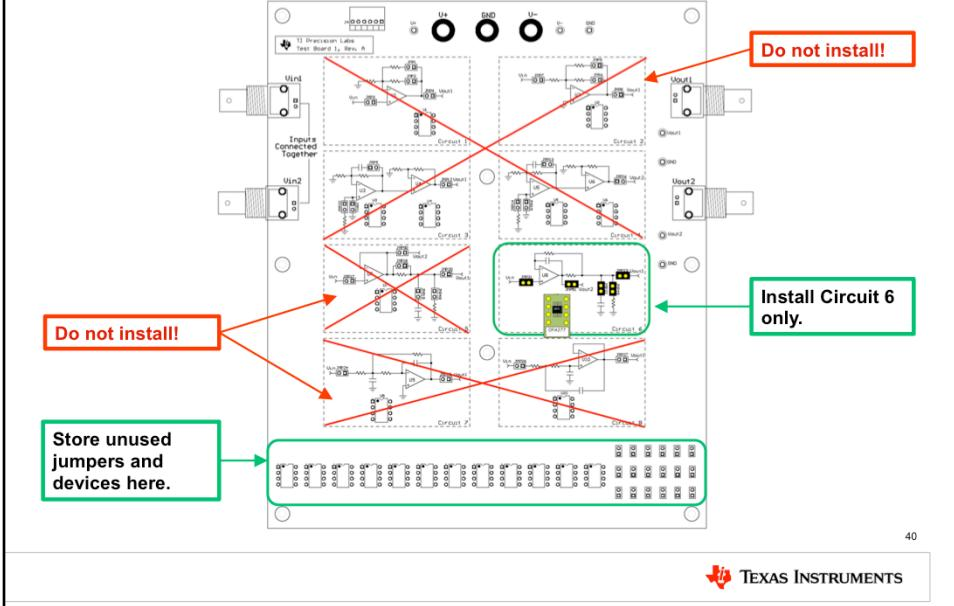
For the test board to function properly, it is important that you only install jumpers and devices in circuit 6! Do not install any jumpers or devices in any other circuits on the PCB! Remove any jumpers or devices from the unused circuits and store them in the storage area at the bottom of the test board.
