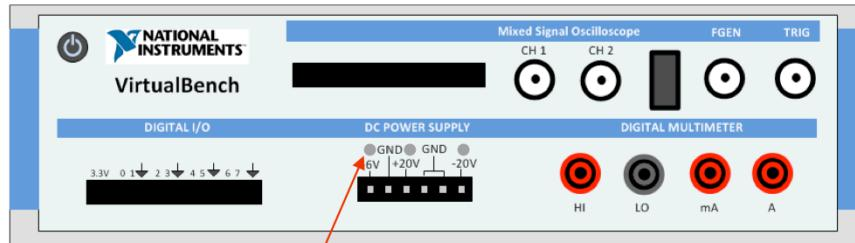
LEDs OFF = DC power supply OFF
