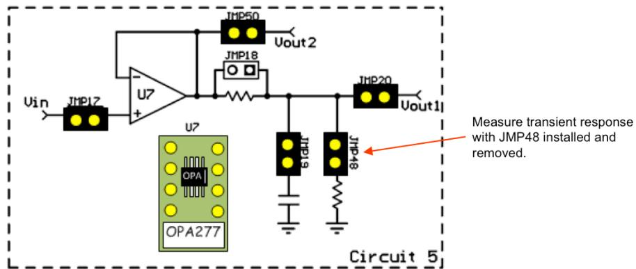
As an additional experiment, measure the transient response again with JMP48 installed and removed. This will connect and disconnect the 1k load resistor from the circuit.
