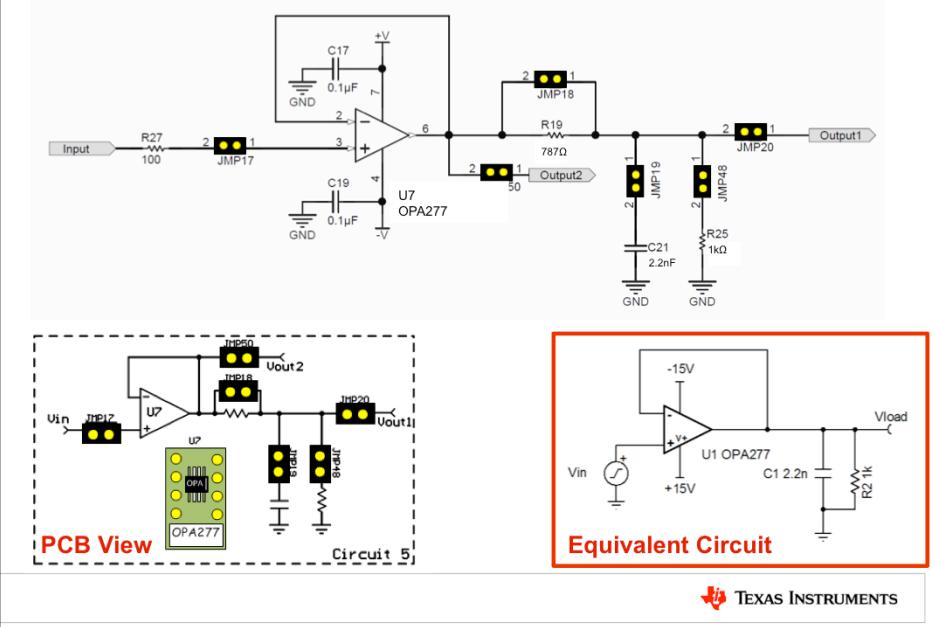
This slide shows the full schematic for Circuit 5 on the TI Precision Labs test board. You will use this circuit to measure the stability of the OPA277.
