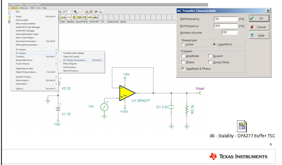
Next, run a SPICE simulation analysis for the AC transfer characteristic. This will allow us to see the op amp's AC peaking, which is another indicator of phase margin.
