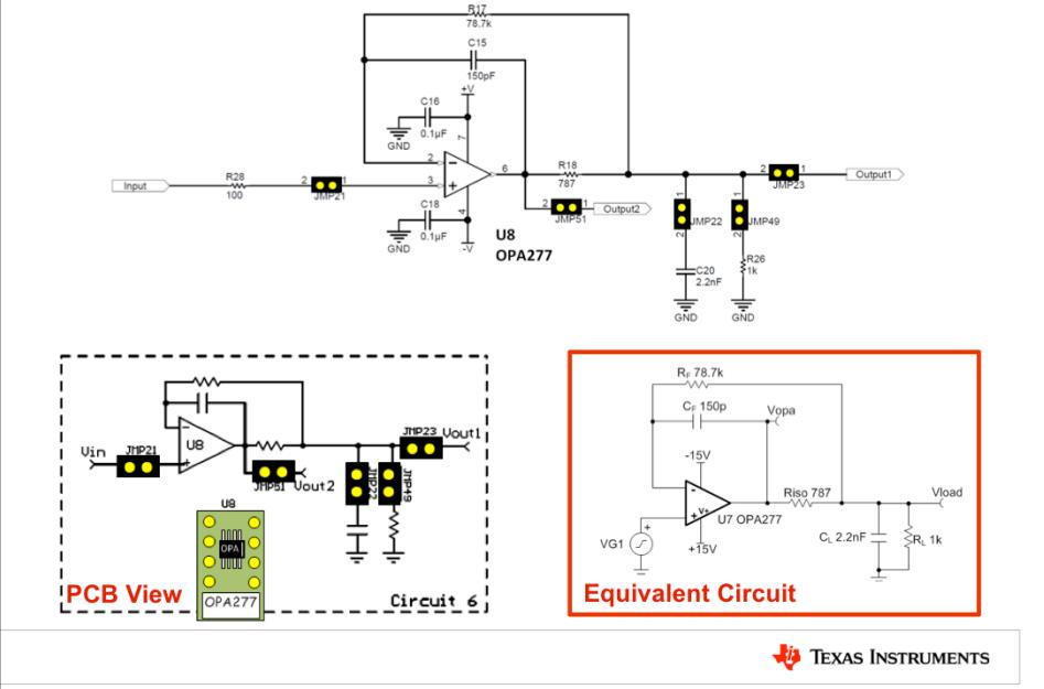
This slide shows the full schematic for Circuit 6 on the TI Precision Labs test board. You will use this circuit to measure the transient behavior of the OPA277 in a dual-feedback configuration.
