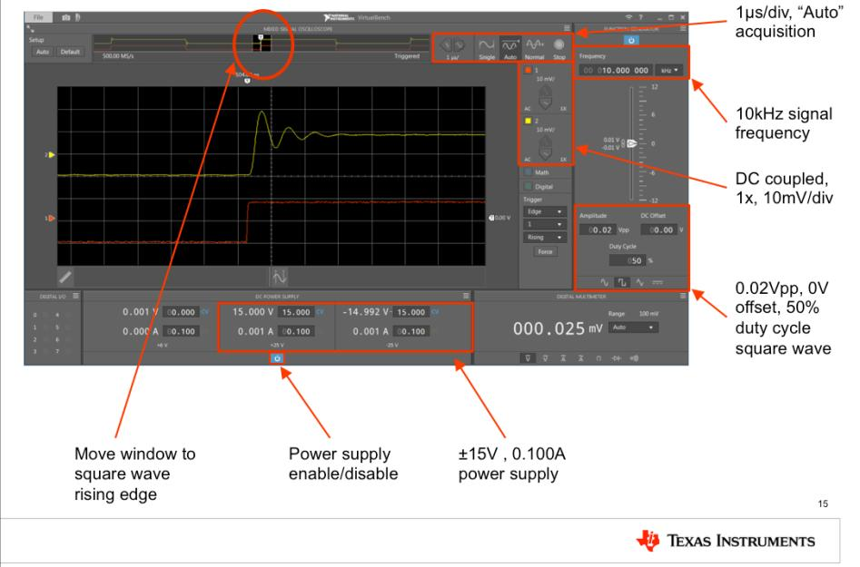
Next apply power to the National Instruments VirtualBench and connect it to your computer with a USB cable. The hardware should be detected as a virtual CD drive, and you can run the VirtualBench software directly from the drive. Once the software opens, configure the software as follows:
