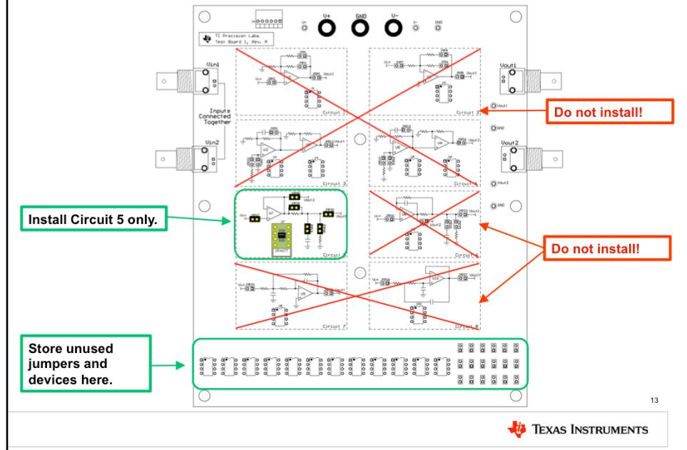
For the test board to function properly, it is important that you only install jumpers and devices in circuit 5. Do not install any jumpers or devices in any other circuits on the PCB! Remove any jumpers or devices from the unused circuits and store them in the storage area at the bottom of the test board.
