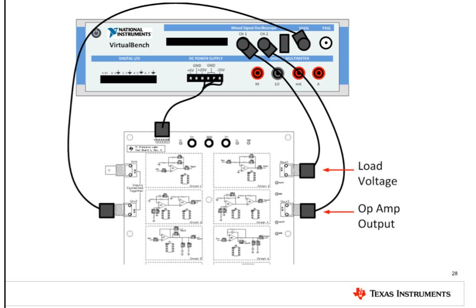
This slide gives the new connection diagram between the TI Precision Labs test board and the National Instruments VirtualBench. Connect the provided power cable to the DC power supply of the Virtual Bench and power connector J4 on the test board.
