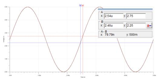
A = 2.5 V F = 400 kHz Max slew rate  $\approx$  6.28 V/ $\mu$ s
